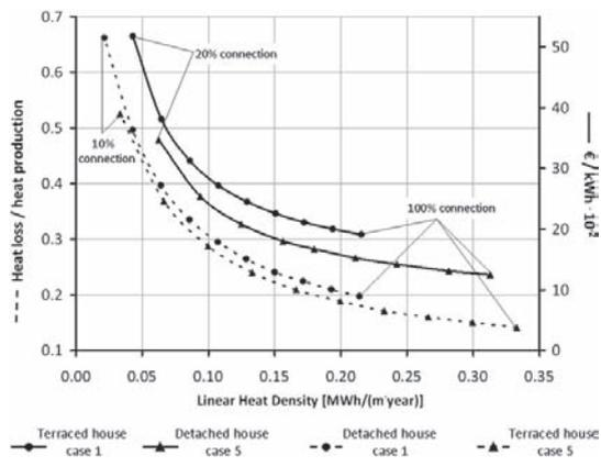
**Fig. 5.** Heat loss/total produced heat vs. the linear heat density (---). Specific energy cost (—). The picture shows the bottom and top curves. All the values are between the top and bottom lines, for all the cases considered.
