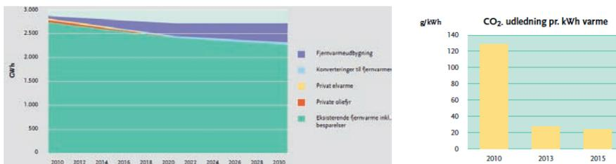
**Heating forecast for AVA based on the Danish Building Code 2010 (left). The CO<sub>2</sub>-emission per produced kWh heat at the main heat exchanger (right).**
