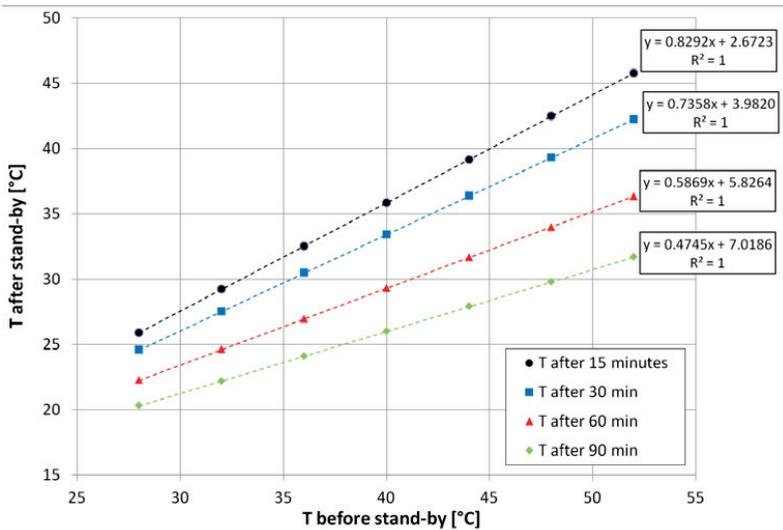
Figure 5.3 Examples of cooling-off curves of the heat carrier, derived by 2-D transient heat transfer simulations in COMSOL Multiphysics. Service pipe: Alx. 20-20/110. At  $\tau=0$  s:  $T_{soil}= 8^{\circ}C$ ,  $T_{PUR}= 15^{\circ}C$ ,  $T_{return}= 25^{\circ}C$ .
