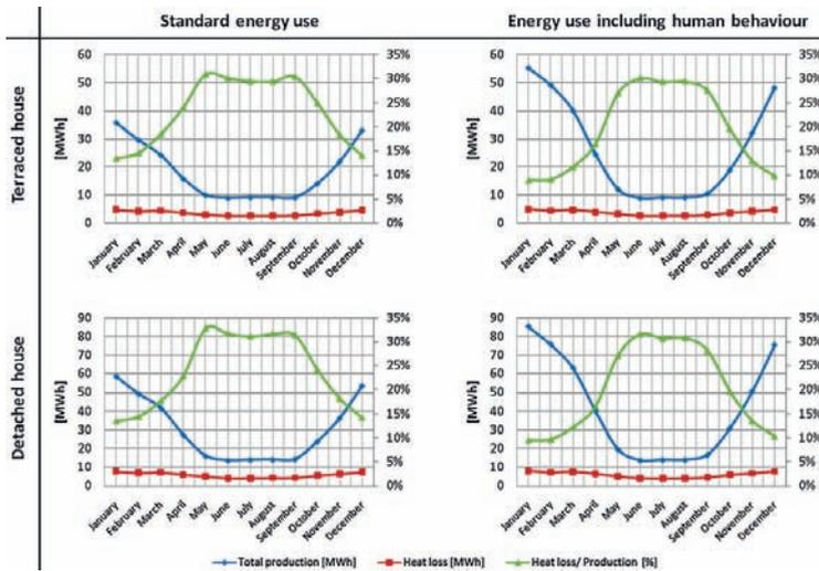
**Fig. 4.** Monthly heat production and heat loss [MWh] and quota distribution heat loss and heat production. DH supply/return temperatures: 55/25 °C. Cases with terraced houses (top); cases with detached houses (bottom). Standard energy use (left); energy use including human behaviour (right).
