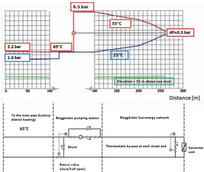
Simplified pressure/temperature diagram of the mixing shunt.
