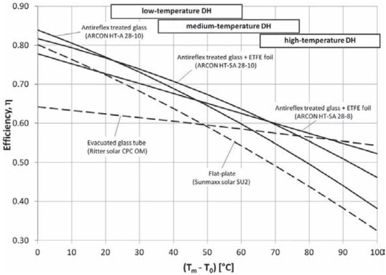
Fig. 3. Efficiency of solar collectors as function of the difference between the average  $T$  of the fluid in the collector,  $T_m$  and the ambient temperature,  $T_0$  ( $G = 1000 \text{ W/m}^2$ ). — Large-scale solar thermal collector, source: [27]; - - - Small-scale solar thermal collector, source: [28].
