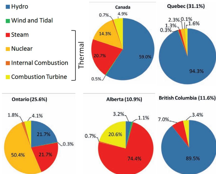
*Figure 5.8 Electricity production by energy source in Canada as a whole and in the main Provinces in 2007. The percentage between brackets indicates the share of the national production, which was equivalent to 2223 PJ. Derived from [57].*
