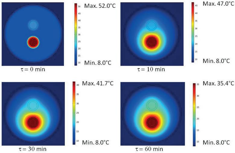
Figure 5.4 Cooling of the water in the supply media pipe of the service pipe during the stand-by period. Example: service pipe: Alx. 20-20/110. At  $\tau=0$  s:  $T_{soil}=8^{\circ}\text{C}$ ,  $T_{PUR}=15^{\circ}\text{C}$ ,  $T_{supply}=52^{\circ}\text{C}$ ,  $T_{return}=25^{\circ}\text{C}$ .
