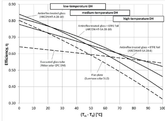
Figure 3.3 Efficiency of solar thermal collectors as function of the difference between the average temperature of the fluid in the collector,  $T_m$  and the ambient temperature,  $T_0$  ( $G = 1000 \text{ W/m}^2$ ). — Large-scale solar thermal collectors, source: [25][24]; ---- Small-scale solar thermal collectors, source: [26].
