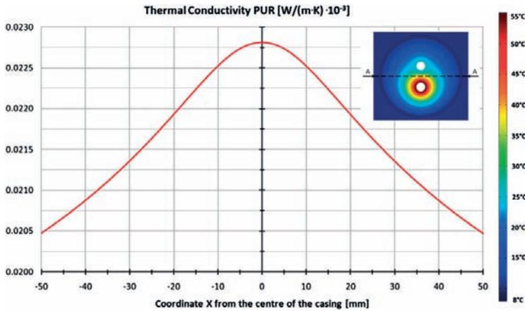
Fig. 3. Thermal conductivity in the insulation, pipe cross-section A–A. Pipe: Aluflex 16–16/110. Temperatures supply/return/ground 55/25/8 °C.
