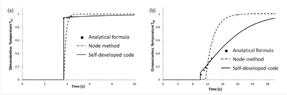
Figure 5: Dimensionless temperature profiles. Step function response. (a): single pipe, steel, DN300; characteristics:  $L = 10\text{m}$ ,  $d = 263\text{ mm}$ ,  $t_{\text{pipe}} = 5\text{ mm}$ ,  $v = 2.71\text{ m/s}$ . (b): twin pipe, aluflex 20-20/110; characteristics:  $L = 10\text{m}$ ,  $d = 15\text{ mm}$ ,  $t_{\text{pipe}} = 2.5\text{ mm}$ ,  $v = 1.00\text{ m/s}$ .
