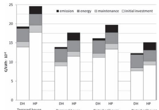
**Fig. 6.** Levelized cost of energy in case of DH supply and HP supply.
