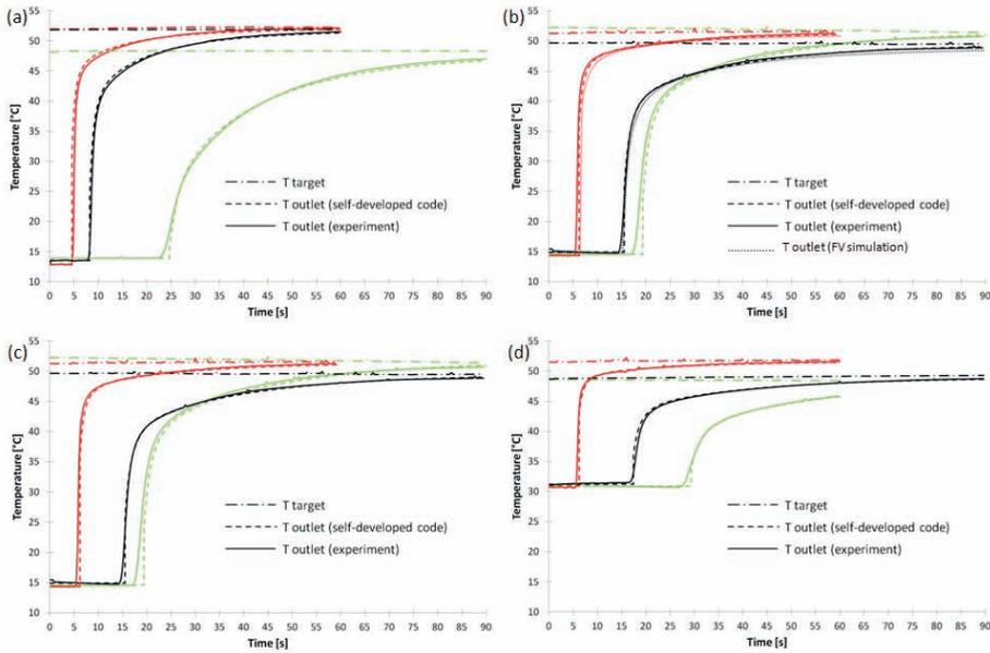
Figure 7: Comparison between the experimental data and the results from simulations with the in-house code. (a): Experiments I-III; (b): experiments IV-VI; (c): experiments VII-IX; and (d): experiments X-XII.
