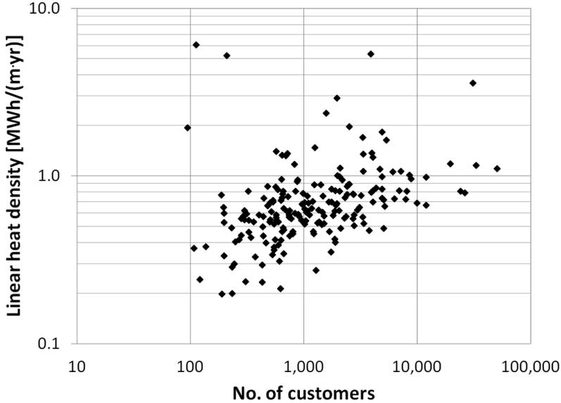
Figure 2.6 Linear heat density vs. number of customers in 200 existing DH networks in Denmark, based on heat use data in 2010. Source: [12].
