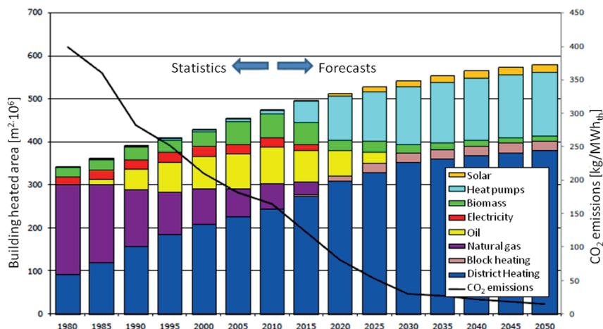
Figure 2.7 Historical data and future projections about total heated area, CO<sub>2</sub> emissions and heat supply for the “rapid development” scenario. Source: [17].
