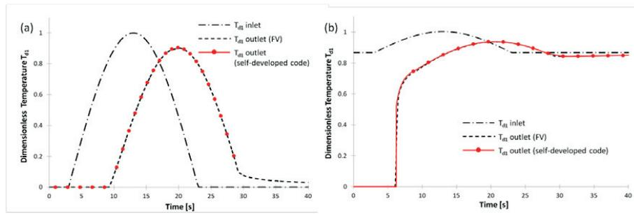
Figure 6: Dimensionless temperature profiles. Sinusoidal function response.  $A = 5^{\circ}\text{C}$ ,  $B = 0.157 \text{ s}^{-1}$ ,  $\tau_{\text{delay}} = 3 \text{ s}$ ,  $T_{\text{water, initial}} = 46.35^{\circ}\text{C}$ . (a):  $T_{\text{inlet, initial}} = 46.35^{\circ}\text{C}$  and (b):  $T_{\text{inlet, initial}} = 14.25^{\circ}\text{C}$ .
