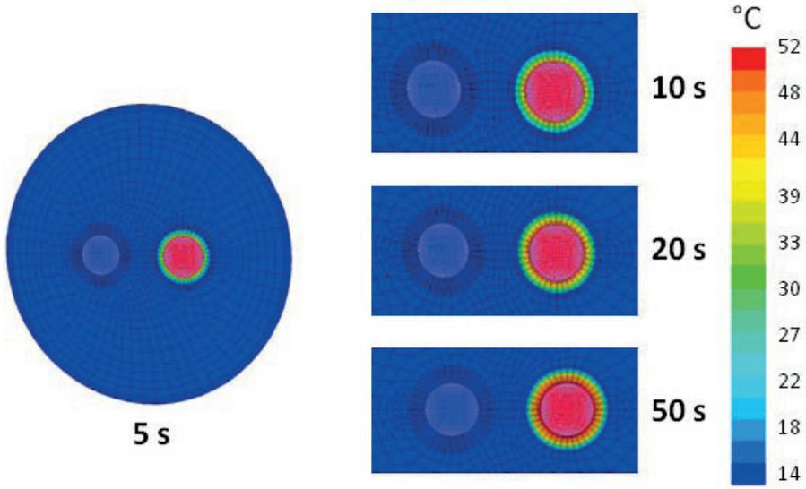
Figure 4: Temperature contour [°C] at the inlet cross section of the media pipe at different transition times. Aluflex 20-20/110,  $T_{\text{supply}} = 51.5^{\circ}\text{C}$ ,  $T_{\text{initial}} = 14.4^{\circ}\text{C}$ ,  $v = 2.36 \text{ m/s}$ .
