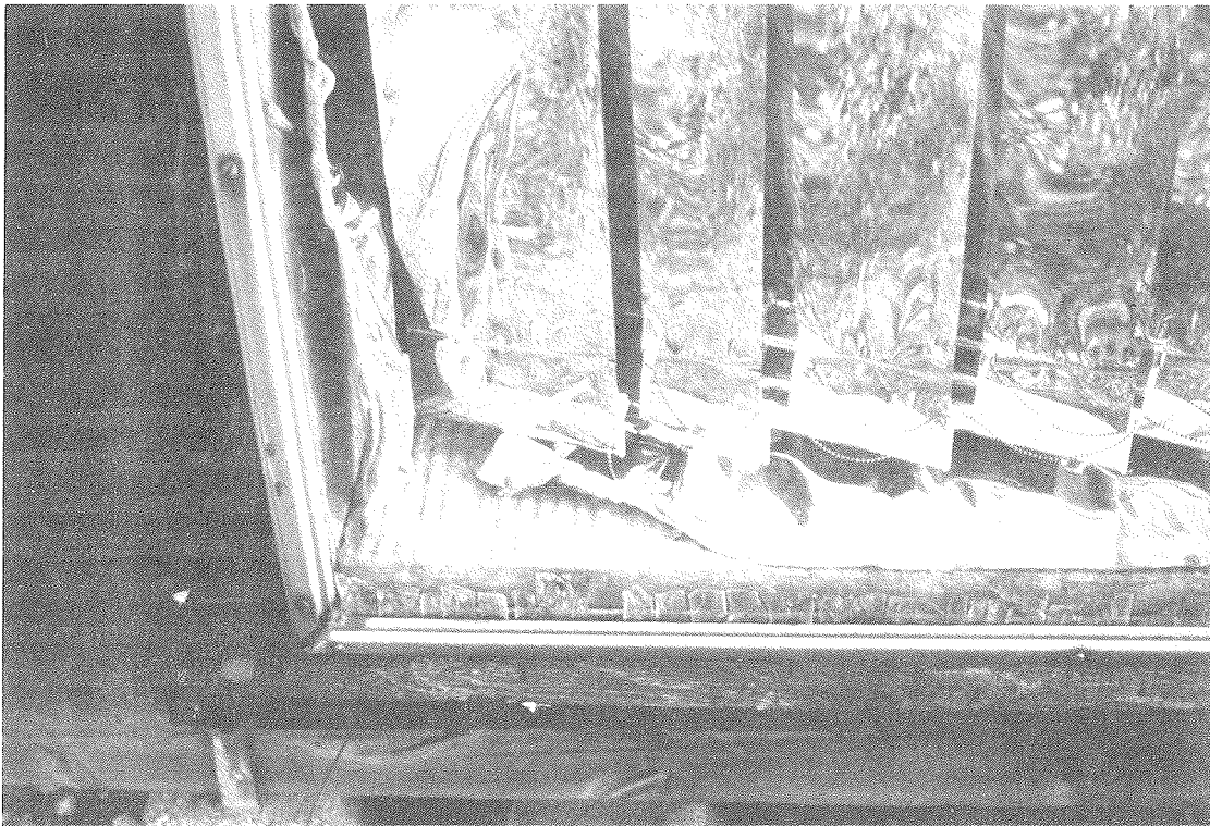
Figure 4.1 The bright adhesive plastic foil on the additional insulation on the thermo laths of wall 1 had after three and a half years lost its adhesive ability and had crumpled up.
