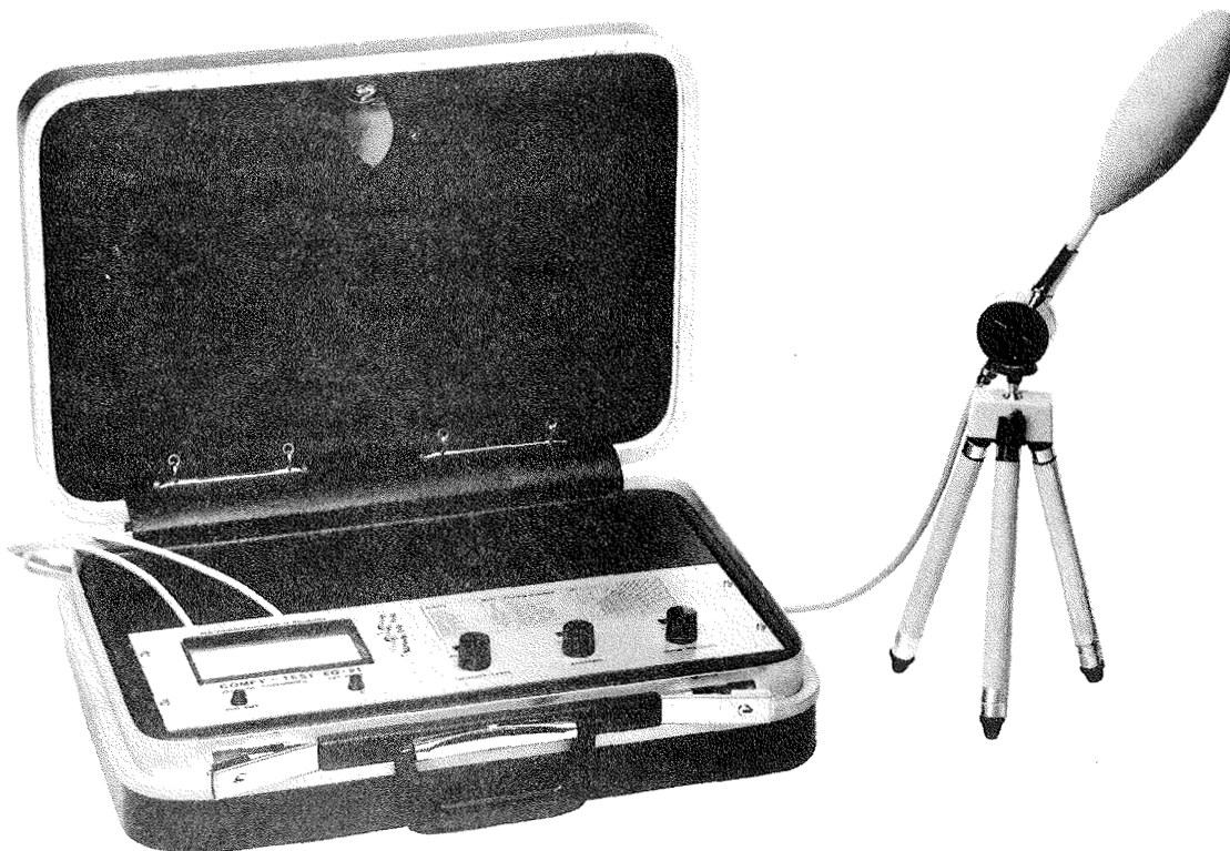
Figure 6. The thermal comfort meter. (Comfy test manufactured by RECI LTD, Copenhagen).
