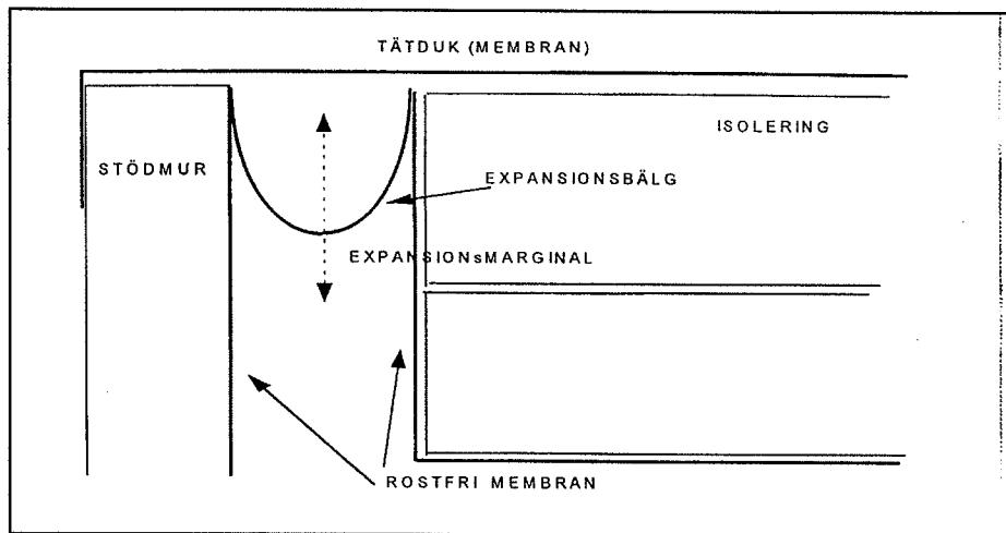
Figure 17 Border design for the Swedish floating lid design.
