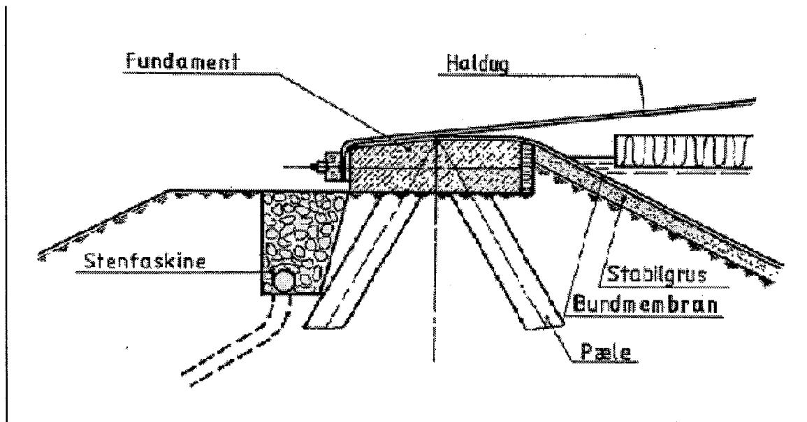
Figure 1 Principal sketch of floating lid border design. Pontoon with insulation.
