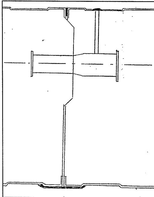
*Figure 10 The assembly details for the sandwich elements. The two elements are fixed by a plastic bolt and the joints sealed by silicone mass and ID-tape.*
