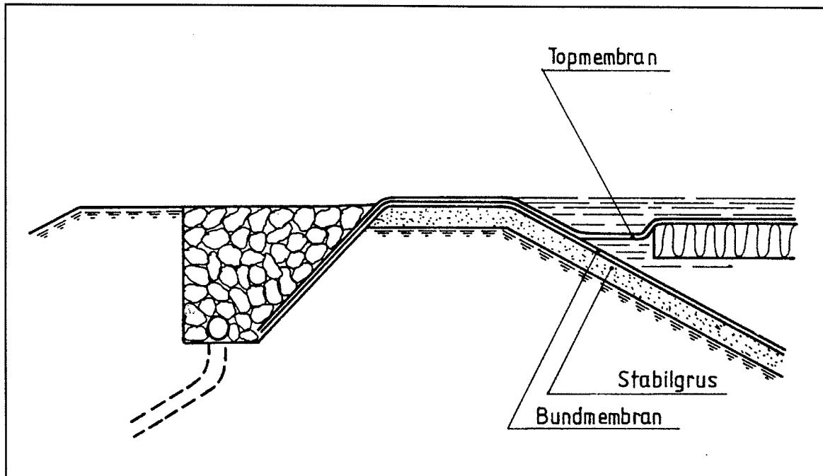
Figure 3 Principal sketch of floating lid border design. Submerged insulation with top membrane.
