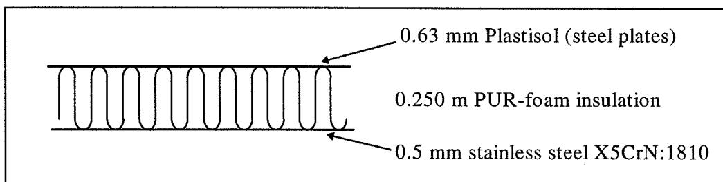
Figure 8 Sandwich element applied to the Ottrupgaard lid. The element is basically two plates filled with PUR foam as insulating material. This composition is rather stiff and stable without any additional stabilising constructions.
