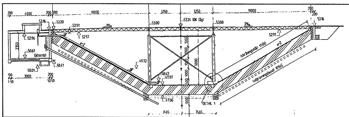
*Figure 7 The Ottrupgaard lid design. Industrially produced sandwich elements with PUR-foam are applied.*
