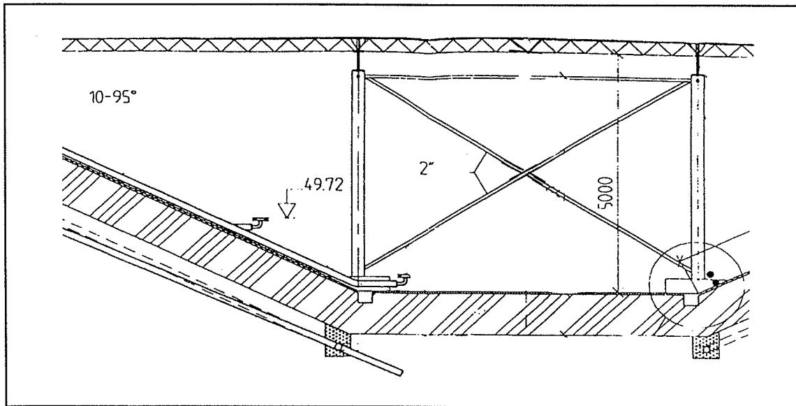
Figure 13 The steel construction supporting the floating lid for the case where no water is in the pit.
