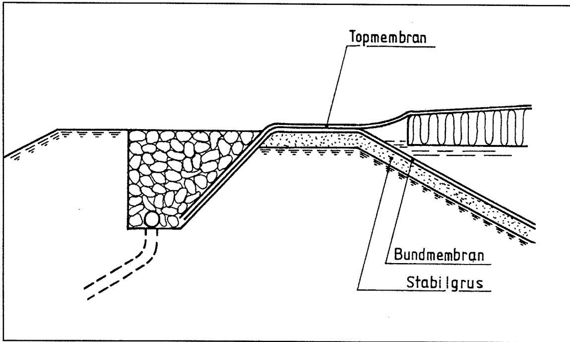
Figure 2 Principal sketch of floating lid border design. Floating insulation with top membrane.
