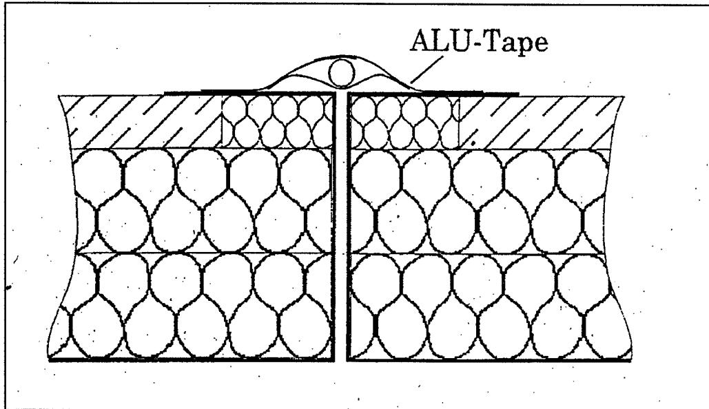
Figure 15 Detail on tightening between pontoons.
