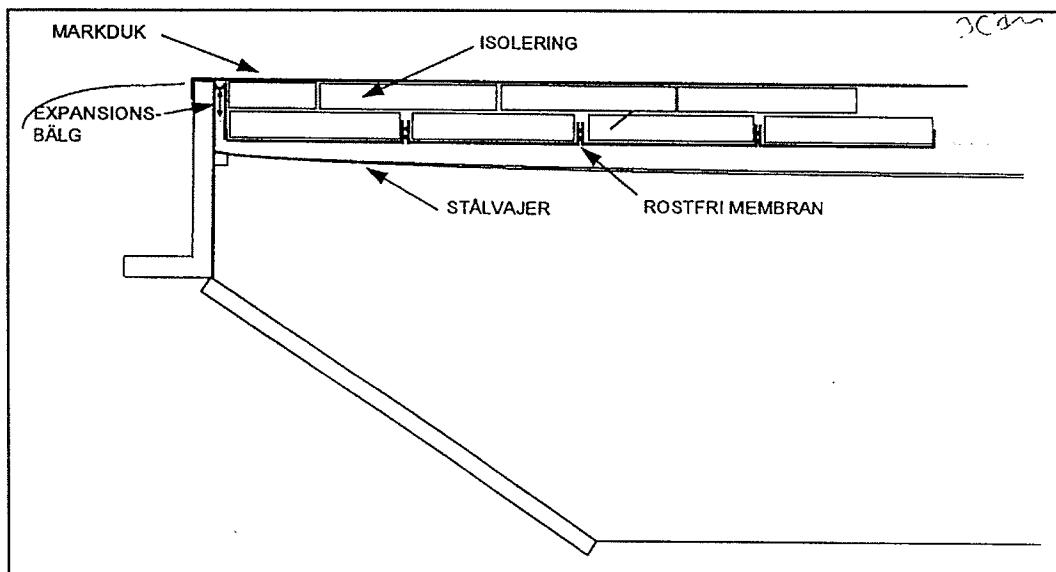
Figure 16 Floating lid construction with U-formed bottom liner.
