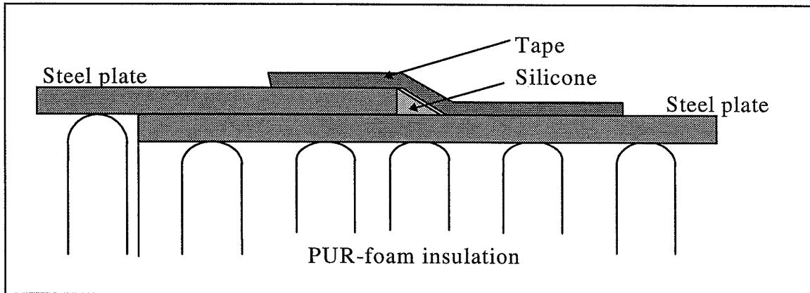
Figure 12 Detail A from Figure 11. The two-step-sealing; a primary sealing of silicone paste and a secondary sealing of a rubber tape which will be discussed in the following sections.
