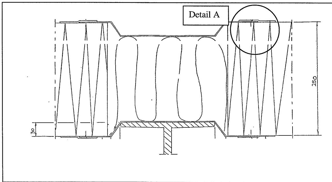
*Figure 11 The assembly details for the sandwich elements. A special joint steel profile is fixed with pop-rivets onto the top- and bottom plate of the two sandwich elements. The joints are tightened by a two-step-sealing, shown in Figure 12. The gap between the elements is then filled with PUR-foam in situ. Note: The I-beam is in contact with the lid only if there is no water in the pit. Otherwise the lid is floating above the steel construction.*
