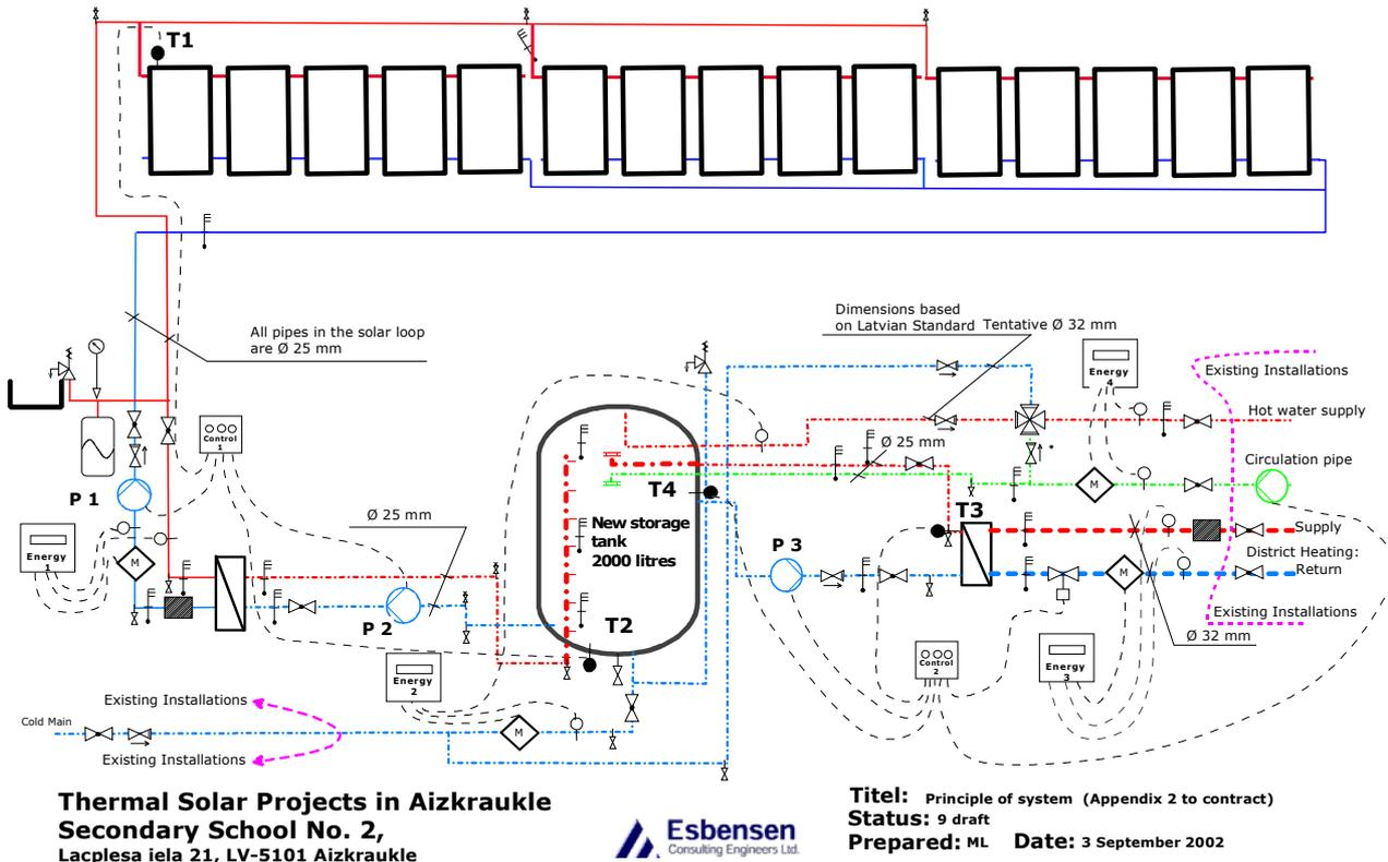
Fig. 3. Schematic illustration of the SDHW system for the school.
