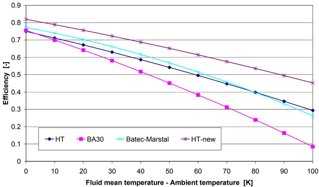
Fig. 10. Efficiency of solar collectors as a function between the mean solar collector fluid temperature and the ambient air temperature.
