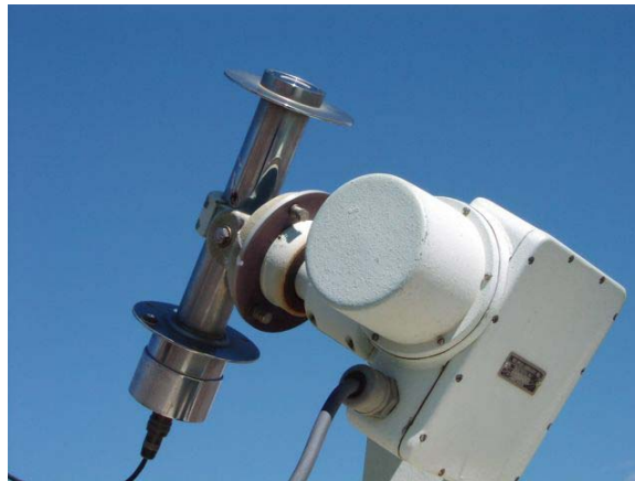
Figure 5: Pyrhelimeter used to measure the solar beam radiation.
