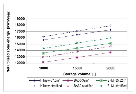
Figure 57: Net utilized solar energy of the solar heating system with about 40  $m^2$  different solar collectors as a function of the storage volume for a tapping profile of 2  $m^3$  for 5 days.
