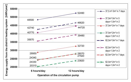
Figure 41: Energy supply from the district heating system as a function of the operating hours of the circulation pump.
