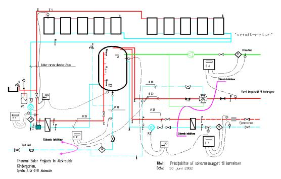
Figure 2: Schematic illustration of the solar heating system for the kindergarten.
