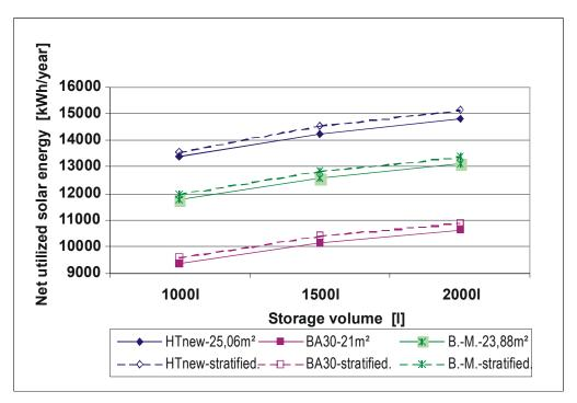
Figure 56: Net utilized solar energy of the solar heating system with about 20  $m^2$  different solar collectors as a function of the storage volume for a tapping profile of 4  $m^3$  for 5 days.
