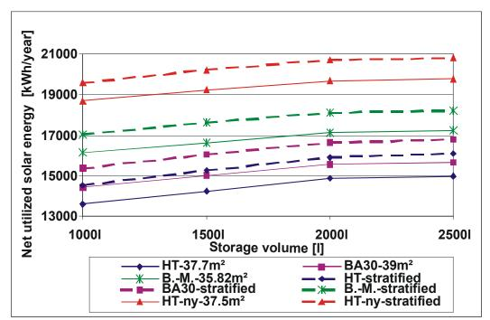
Figure 27: Net utilized solar energy of the solar heating system with about 40 m<sup>2</sup> different solar collectors as a function of the storage volume for a tapping profile of 2 m<sup>3</sup> for 5 days + 1.0 m<sup>3</sup> for 2 days.
