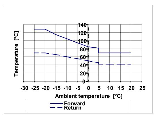
Figure 4: Temperature level for Aizkraukle's district heating system.
