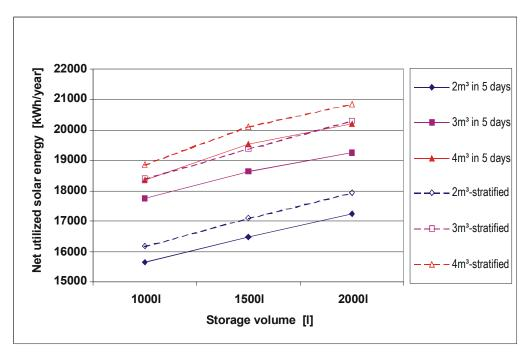
Figure 49: Net utilized solar energy as a function of the storage volume for the system with 37.5  $m^2$  new HT solar collectors.
