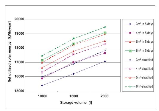
Figure 44: Net utilized solar energy as a function of the storage volume for the system with 35.82 m<sup>2</sup> B.-Marstal solar collectors.
