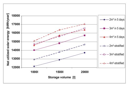
Figure 53: Net utilized solar energy as a function of the storage volume for the system with 39  $m^2$  BA30 solar collectors.
