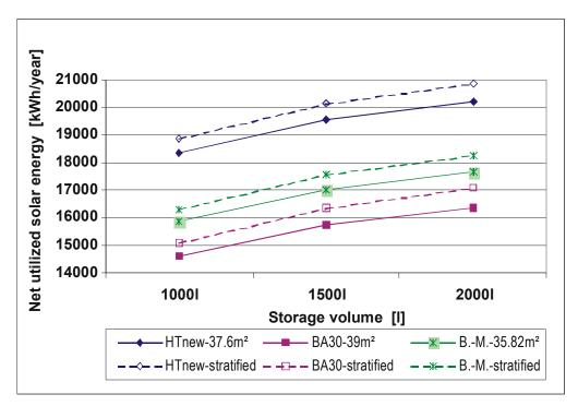
Figure 59:Net utilized solar energy of the solar heating system with about 40  $m^2$  different solar collectors as a function of the storage volume for a tapping profile of 4  $m^3$  for 5 days.
