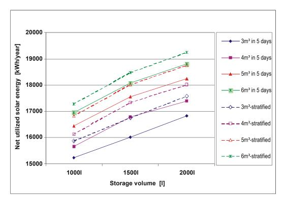
Figure 42: Net utilized solar energy as a function of the storage volume for the system with  $37.5 \text{ m}^2 \text{HT}$  solar collectors.
