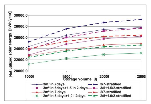
Figure 21: Net utilized solar energy as a function of the storage volume for the system with a  $62.5 \text{ m}^2 \text{ HT}$  solar collector.
