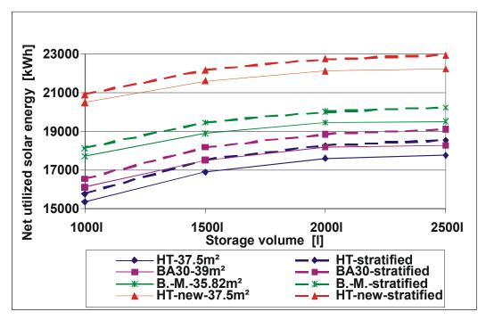
Figure 24: Net utilized solar energy of the solar heating system with about 40  $m^2$  different solar collectors as a function of the storage volume for the tapping profile of 3  $m^3$  for 7 days.
