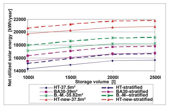
Figure 26: Net utilized solar energy of the solar heating system with about 40 m<sup>2</sup> different solar collectors as a function of the storage volume for a tapping profile of 3 m<sup>3</sup> for 5 days + 1.5 m<sup>3</sup> for 2 days.
