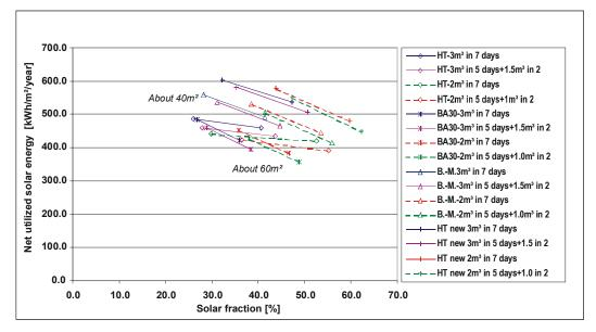
Figure 33: The net utilized solar energy of the solar heating system as a function of the solar fraction for different solar collectors and solar collector areas (2000 I storage with stratified inlet from the solar collector loop).
