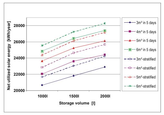
Figure 43: Net utilized solar energy as a function of the storage volume for the system with 62.5  $m^2$  HT solar collectors.
