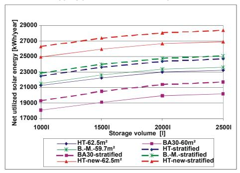
Figure 31: Net utilized solar energy of the solar heating system with about 60 m<sup>2</sup> different solar collectors as a function of the storage volume for a tapping profile of 2 m<sup>3</sup> for 5 days+1.0 m<sup>3</sup> for 2 days.
