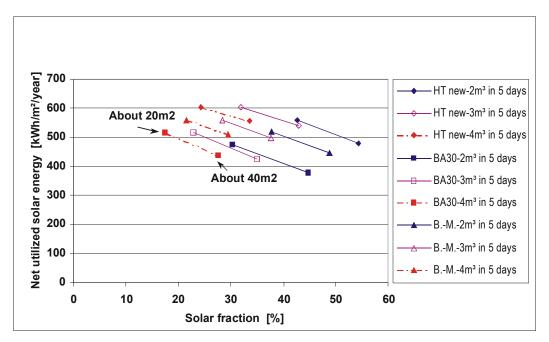
Figure 61: The utilized solar energy of the solar heating system as a function of the solar fraction for different solar collectors and solar collector areas (2000 I storage with stratified inlet from the solar collector loop).
