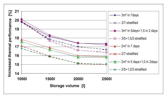
Figure 39: Increase of the thermal performance of the solar heating system (with about 60  $m^2$  solar collectors) by using the new HT solar collector instead of the old HT solar collector.
