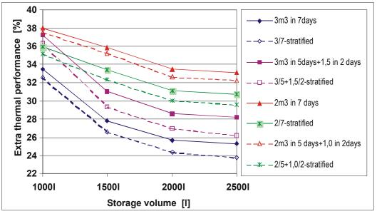
Figure 38: Increase of the performance of the solar heating system (with about 40  $m^2$  solar collectors) by using the new HT solar collector instead of the old HT solar collector.
