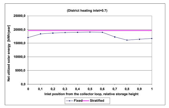
Figure 14: The thermal performance of the solar heating system as a function of the inlet position from the solar collector loop with about  $40 \text{ m}^2$  solar collector area and a tapping profile of 3 m<sup>3</sup> for 7 days.
