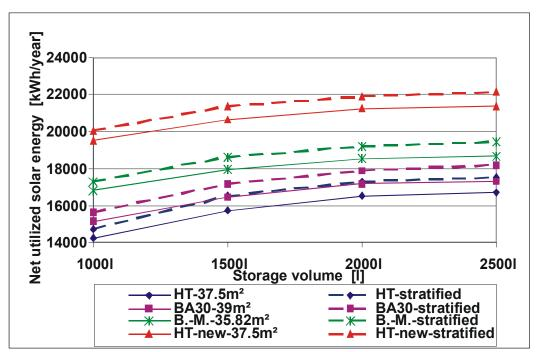
Figure 25: Net utilized solar energy of the solar heating system with about 40 m<sup>2</sup> different solar collectors as a function of the storage volume for a tapping profile of 3 m<sup>3</sup> for 7 days + 1.5 m<sup>3</sup> for 2 days.
