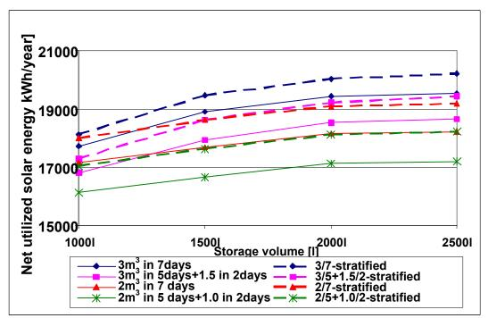
Figure 18: Net utilized solar energy as a function of the storage volume for the system with a 35.82 m<sup>2</sup> Batec-Marstal solar collector.
