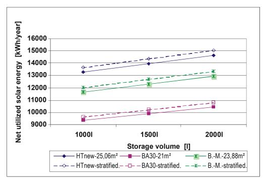
Figure 55: Net utilized solar energy of the solar heating system with about 20 m<sup>2</sup> different solar collectors as a function of the storage volume for a tapping profile of 3 m<sup>3</sup> for 5 days.
