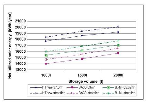
Figure 58: Net utilized solar energy of the solar heating system with about 40  $m^2$  different solar collectors as a function of the storage volume for a tapping profile of 3  $m^3$  for 5 days.
