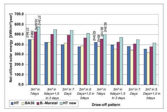
Figure 35: The net utilized solar energy of the solar heating system per  $m^2$  solar collector as a function of the consumption pattern for different solar collectors with 1500 l storage.
