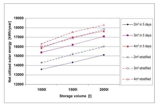
Figure 51: Net utilized solar energy as a function of the storage volume for the system with 35.82 m<sup>2</sup> B.-Marstal solar collectors.
