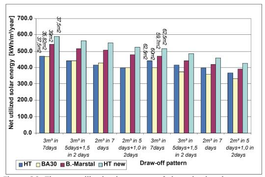
Figure 36: The net utilized solar energy of the solar heating system per  $m^2$  solar collector as a function of the consumption pattern for different solar collectors with 2000 l storage.
