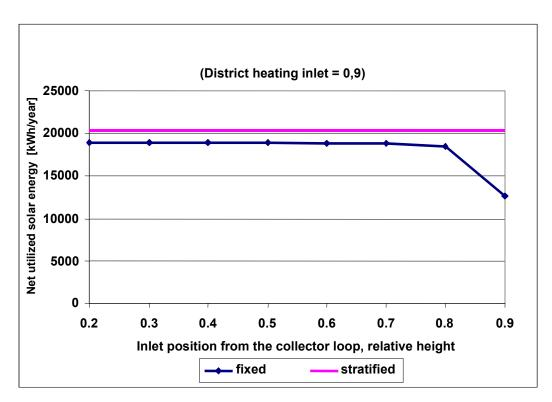
Figure 15: The performance of the solar heating system as a function of the inlet position from the solar collector loop with about 60  $m^2$  solar collector area and a tapping profile of 2  $m^3$  for 5 days+1.0  $m^3$  for 2 days.
