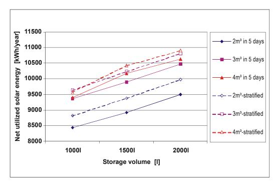
Figure 52: Net utilized solar energy as a function of the storage volume for the system with 21  $m^2$  BA30 solar collectors.
