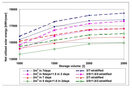
Figure 17: Net utilized solar energy as a function of the storage volume for the system with a 37.5  $m^2$  HT solar collector.
