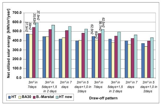
Figure 37: The net utilized solar energy of the solar heating system per  $m^2$  solar collector as a function of the consumption pattern for different solar collectors with 2500 l storage.
