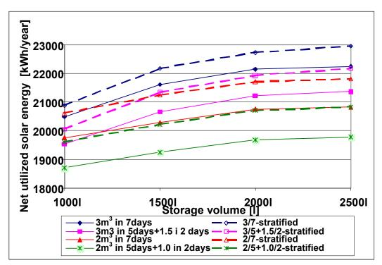
Figure 20: Net utilized solar energy as a function of the storage volume for the system with a 37.5m<sup>2</sup> HT-new solar collector.
