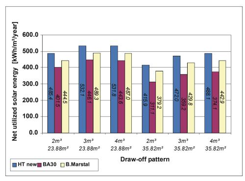
Figure 62: The net utilized solar energy of the solar heating system per  $m^2$  solar collector as a function of the consumption pattern for different solar collectors with 1000 l storage.
