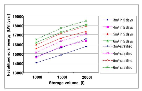
Figure 46: Net utilized solar energy as a function of the storage volume for the system with 39  $m^2$  BA30 solar collectors.
