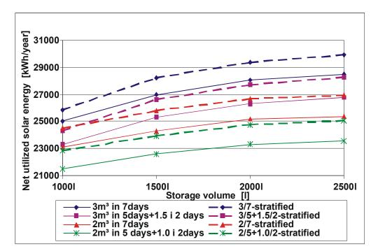
Figure 22: Net utilized solar energy as a function of the storage volume for the system with a 59.7 m<sup>2</sup> Batec-Marstal solar collector.
