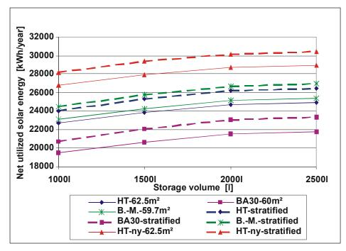
Figure 30: Net utilized solar energy of the solar heating system with about 60  $m^2$  different solar collectors as a function of the storage volume for a tapping profile of 2  $m^3$  for 7 days.
