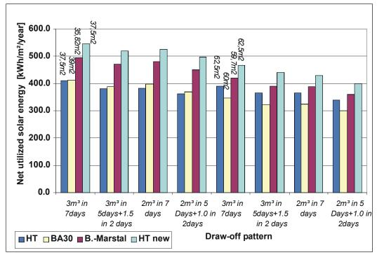
Figure 34: The net utilized solar energy of the solar heating system per  $m^2$  solar collector as a function of the consumption pattern for different solar collectors with 1000 l storage.
