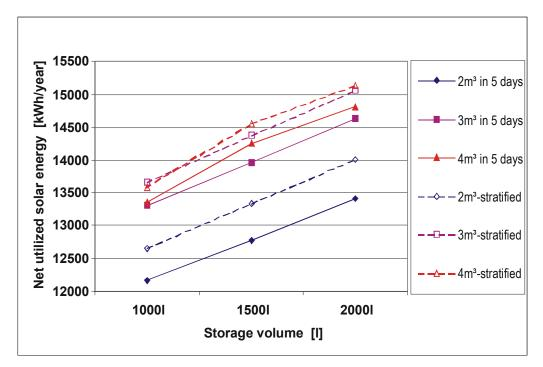
Figure 48: Net utilized solar energy as a function of the storage volume for the system with 25  $m^2$  new HT solar collectors.
