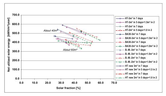
Figure 32: The net utilized solar energy of the solar heating system as a function of the solar fraction for different solar collectors and solar collector areas (2000 I storage with fixed inlet from the solar collector loop).
