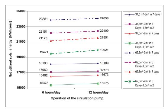
Figure 40: The net utilized solar energy of the solar heating system as a function of the operating hours of the circulation pump.
