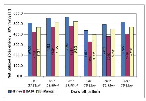
Figure 63: The net utilized solar energy of the solar heating system per  $m^2$  solar collector as a function of the consumption pattern for different solar collectors with 1500 l storage.
