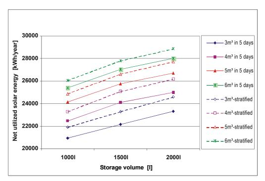
Figure 45: Net utilized solar energy as a function of the storage volume for the system with 59.7 m<sup>2</sup> B.-Marstal solar collectors.
