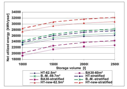
Figure 29: Net utilized solar energy of the solar heating system with about 60 m<sup>2</sup> different solar collectors as a function of the storage volume for a tapping profile of 3 m<sup>3</sup> for 5 days + 1.5 m<sup>3</sup> for 2 days.
