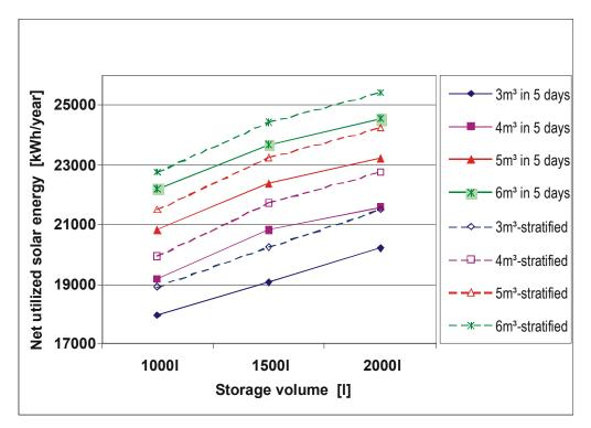
Figure 47: Net utilized solar energy as a function of the storage volume for the system with 60  $m^2$  BA30 solar collectors.
