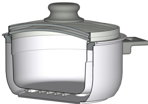
Figure 4. Section view of EffiCooker
