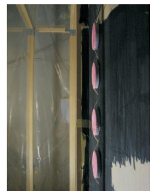
Shallow petri dishes filled with desiccant and with (pink) paper as lid were used to measure the surface moisture transfer coefficient.
