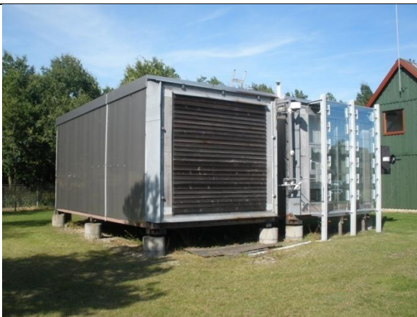
Outdoor test cells for test of hygrothermal room performance and test of daylight control systems
