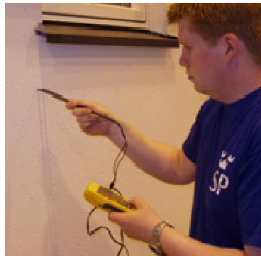
FIG 9. Inserting insulated probes in an upward direction through the holes and through the external insulation.
