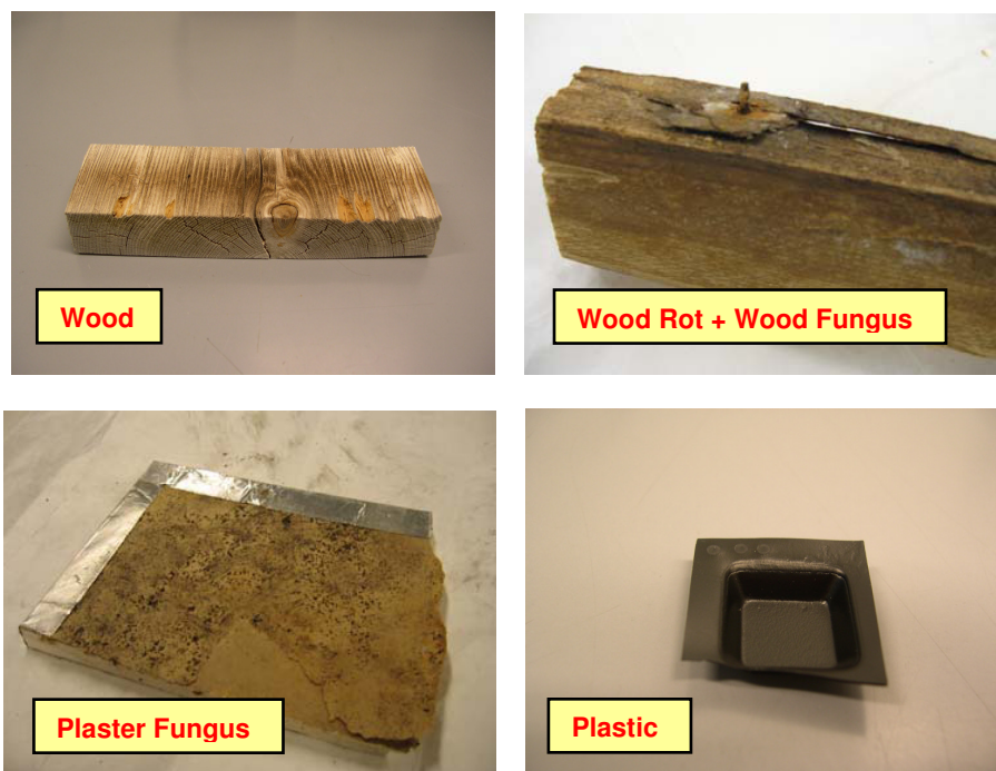
FIG. 1. Photos of the Wood, Wood Rot, Wood Fungus, Plaster Fungus and Plastic samples. Small pieces are cut from the samples for use in the FTIR investigations, except the Plastic sample which is used directly.
