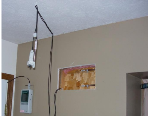
FIG. 5: Data logger and sensor locations in the Kearney wall
