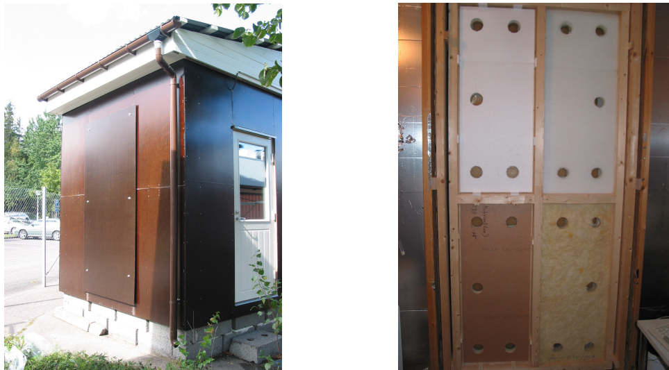
FIG. 4: The test building (on the left) and the wall module which is divided into four different exterior wall assemblies (on the right).
