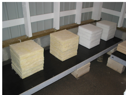
FIG. 2: The small specimens are placed on the steel shelves (on the left) and the piled specimens are palced on the platforms (on the right).
