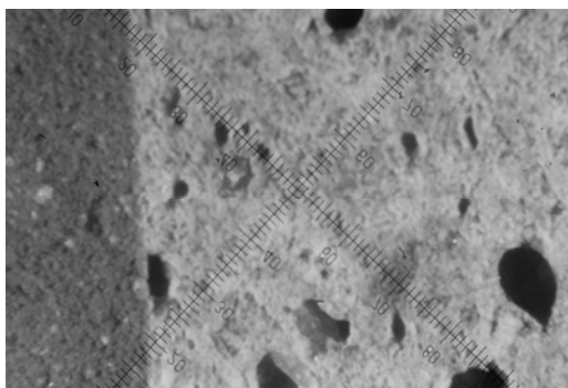
FIG. 7. Images (magnification \times 15 ) of interface between brick and wet cured mortar (left) and brick and dry cured mortar (right).
