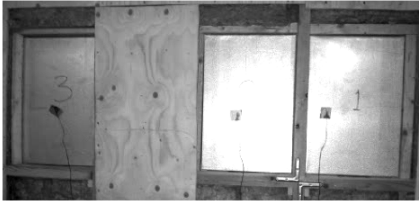
FIGURE 3. The cold side of the climate chamber, with thermometers on the wall cassettes.
