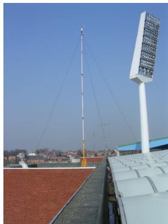
Figure 4: Reference measurement with a 3D ultrasonic anemometer elevated 10 m above the roof of stand 1 of the stadium.
