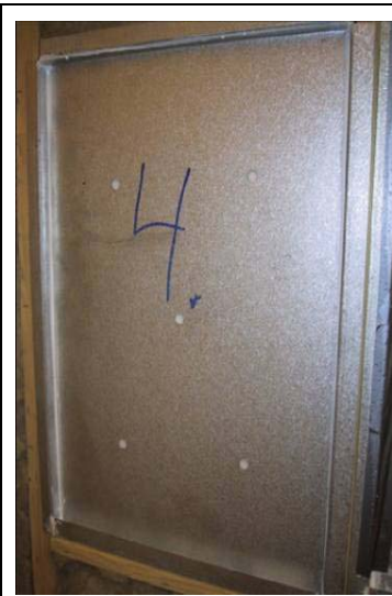
Figure 8. Wall cassette with 5 holes, 3,2 ‰ of total surface.
