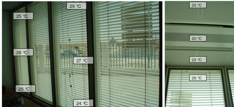
FIG.5: Surface temperature of the glass at the inside and ceiling temperature
