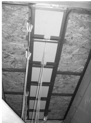
FIG.3: Hot side of the test roof element – heat flux measuring films and PT 1000.
