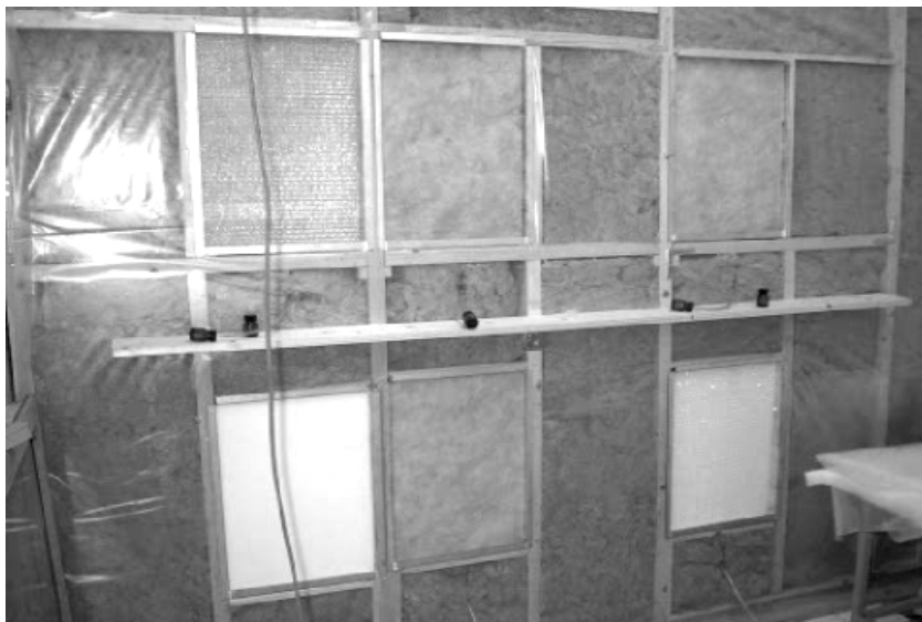
FIGURE 4. The wall cassettes shown from the warm side of the climate chamber.
