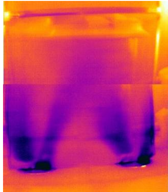
Figure 6 Right . Thermal image of air jet from two adjacent swirl diffusers in the office space. Left . Photo of the set-up.
