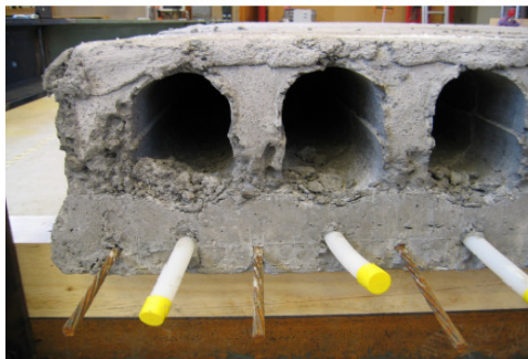
FIG. 1: View of the hollow core concrete deck in which the TABS is integrated
