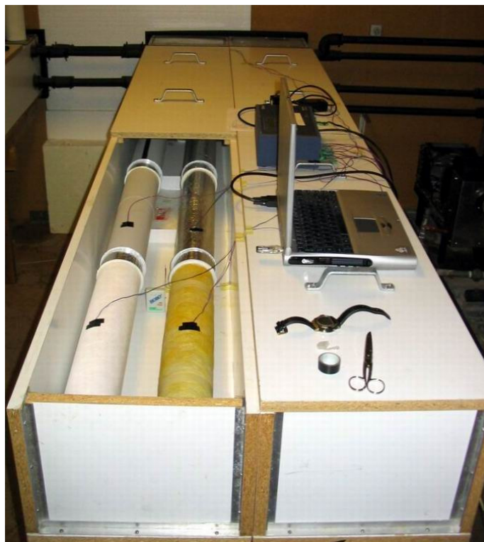
FIG. 2: Configuration of the horizontal and the vertical environmental chamber.
