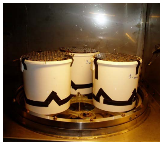
FIG. 6: Section of bucket used for determination of water vapour resistance (left) and photo of buckets in climatic chamber (right).
