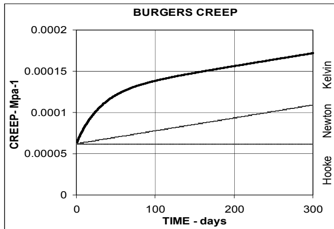
Figure 4. Burgers creep function: E = 16000 \text{ MPa} , \eta = 6.4 * 10^6 \text{ MPa*day} , E_K = 16000 \text{ MPa} , \eta_K = 4.8 * 10^5 \text{ MPa*day} .
