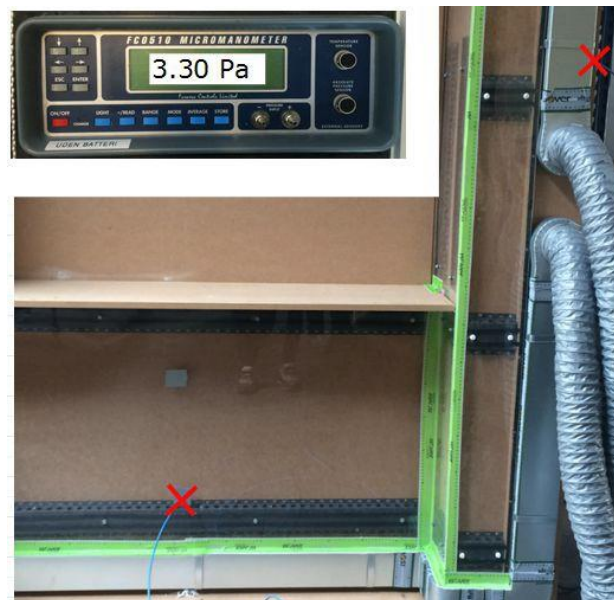
Figure 52: Pressure drop measurement of mock-up model
