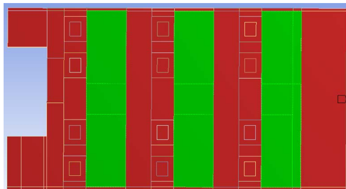
Figure 10: Layout of scenario with reduced area of diffuse ceiling inlet
