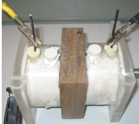
Figure 3: The electrokinetic desalination set-up.
