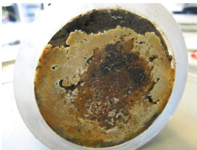
Figure 2: Cathode end of the soil sample after EDR on Soil 2, when the cation-exchange membrane was removed.
