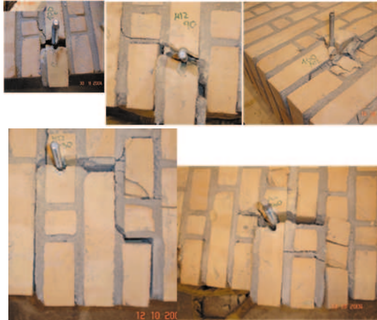
Figure 2.11: Typical splitting failures in masonry
