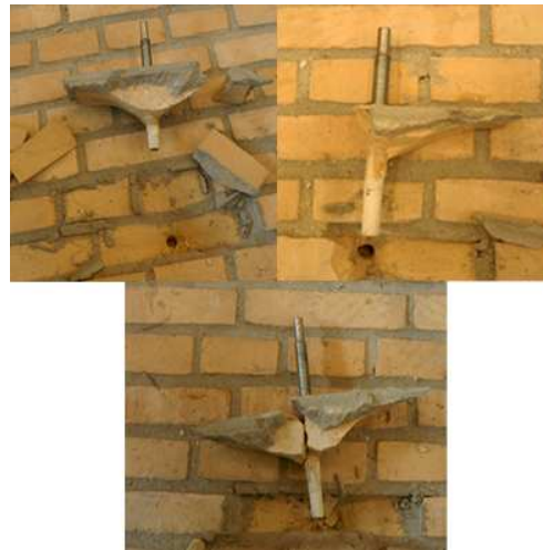
Figure 2.8: Brick-cone failures typically observed in masonry
