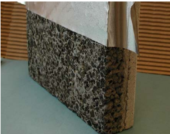
Light weight aggregate concrete with stucco
