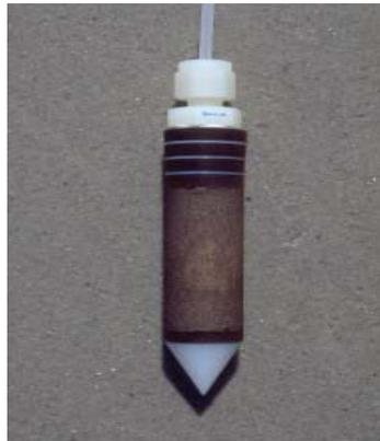
*Figure 11: The Prenart super quartz mini soil solution sampler (from Prenart, 2001)*
