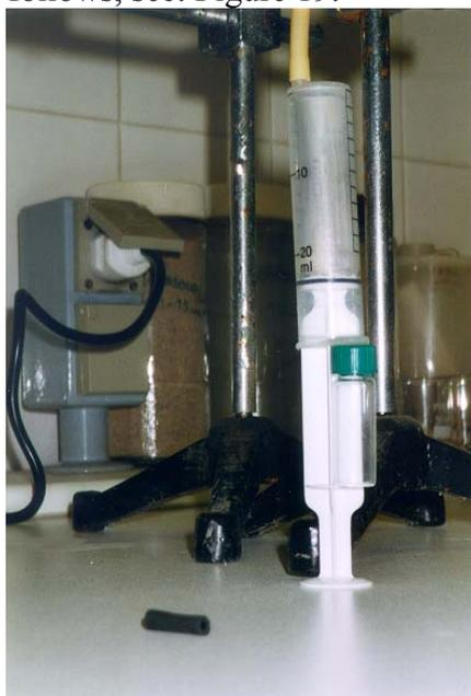
Figure 19: The sampling method for soil solution sampling
