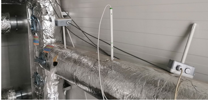
Fig. 5.5: Two combined humidity and temperature sensors and one anemometer for air property measurements (left); Agilent data logging equipment with analogue data logging cards (right).
