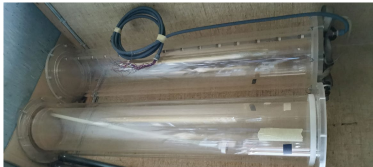
Fig. 5.7: Example for integration of an transparent Plexiglas-pipe with three junctions - currently used in another project (left); two plexiglas pipes with flanges on stock - 1500 x 240 mm, (right).
