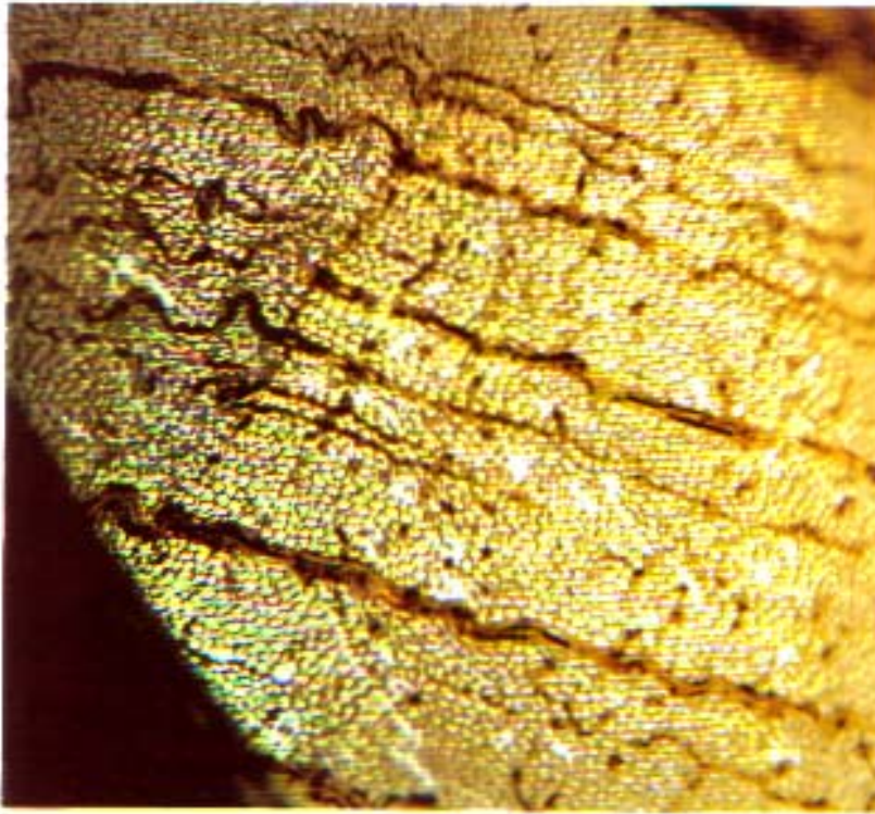
Figure B.1 Compressed beech, C_s=30\% in dry state, magnification 100 X.
