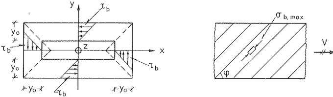
Shear stresses in a cross-section      Concrete stresses at the surface of the beam.
