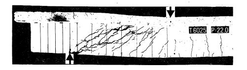
Figure 5: Shear failure of beam with web reinforcement (BRÆSTRUP et al. [6]).
