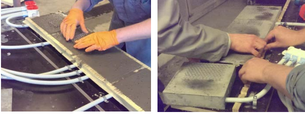
Fig. 2. Production process of concrete blocks with integrated temperature sensors
