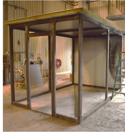
Figure 2.9: a) Placement of the pressure probes with thermocouples along the height of the door and b) Picture of the 1:1 scale SW compartment (E30) post experiment with the back wall and ceiling still attached.
