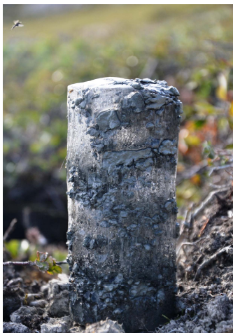
Figure 14: Ice-rich permafrost sample, 26 cm long, extracted from the depth between 1.19 - 1.45 m ca. 20 m east of the ERT profile. Back-lit photo highlights presence of nearly pure ice at the top of permafrost (photo: L. Lindhardt Pedersen).
