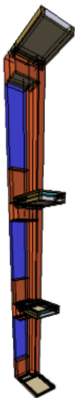
Figure 55 Simulation setup for models without partition wall: Model cut at symmetry line with identical models on top/bottom for boundary conditions.
