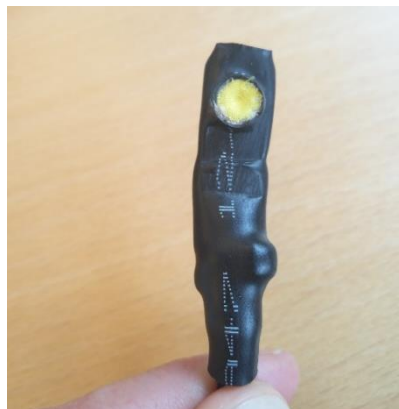
Figure 89 Finished protected sensor and cable connection. Yellow net was covered with cardboard during heating, to avoid glue covering the sensor area.
