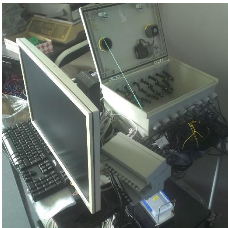
Figure 90 Set-up for calibration: Isolated box with various known salt solutions.
