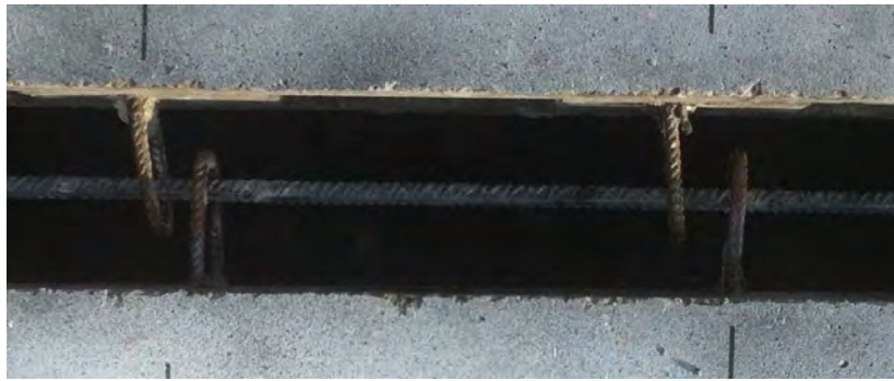
(a) U-bars pushed away from each other (Specimen R1)
