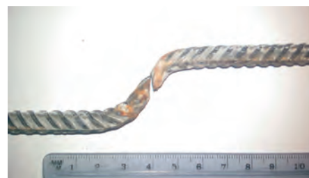
(b) Rupture of rebar
