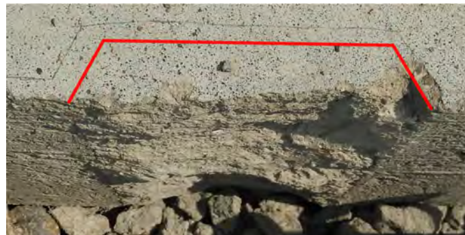
(a) Complete key cut off, Specimen D20B
