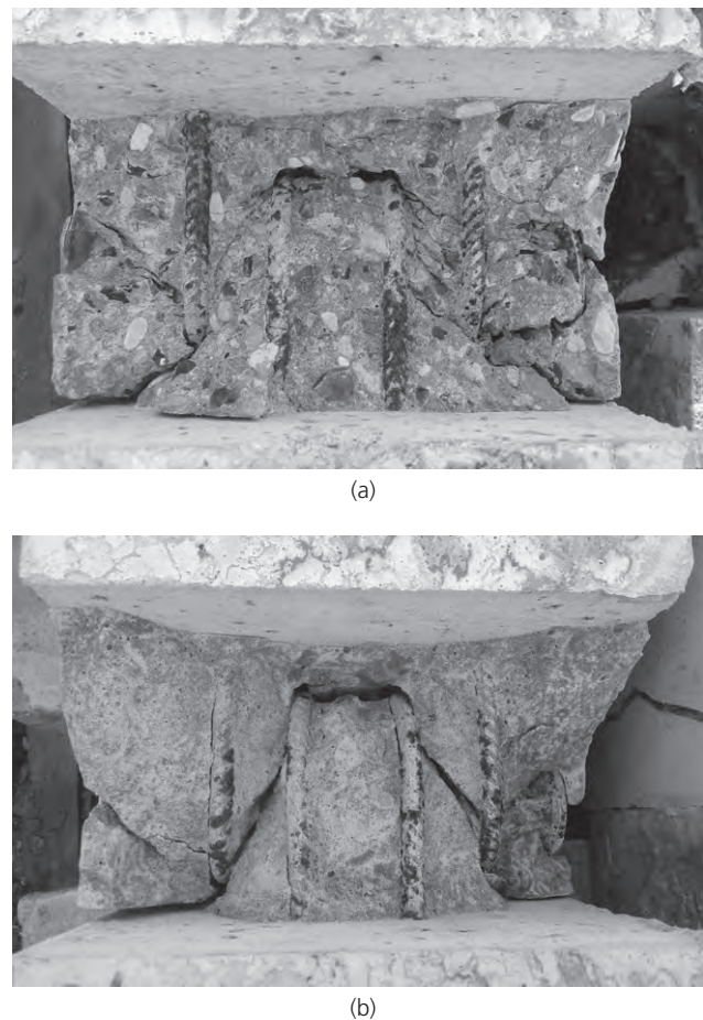
Figure 7. Examples of failed specimens after test: (a) concrete grout (b) mortar grout
