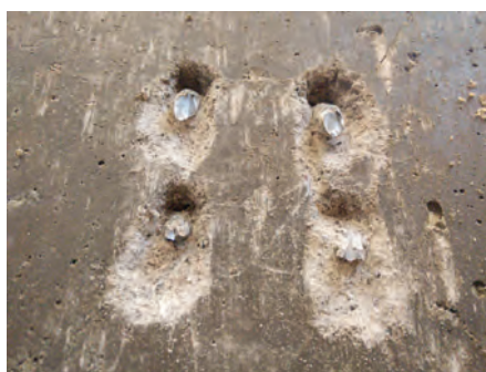
(a) Local crushing of mortar/concrete
