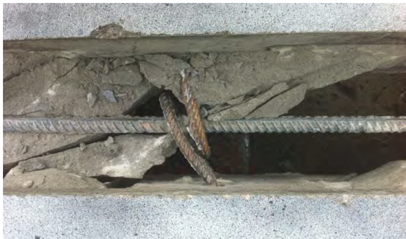
(b) U-bars pushed towards each other (Specimen R6)
