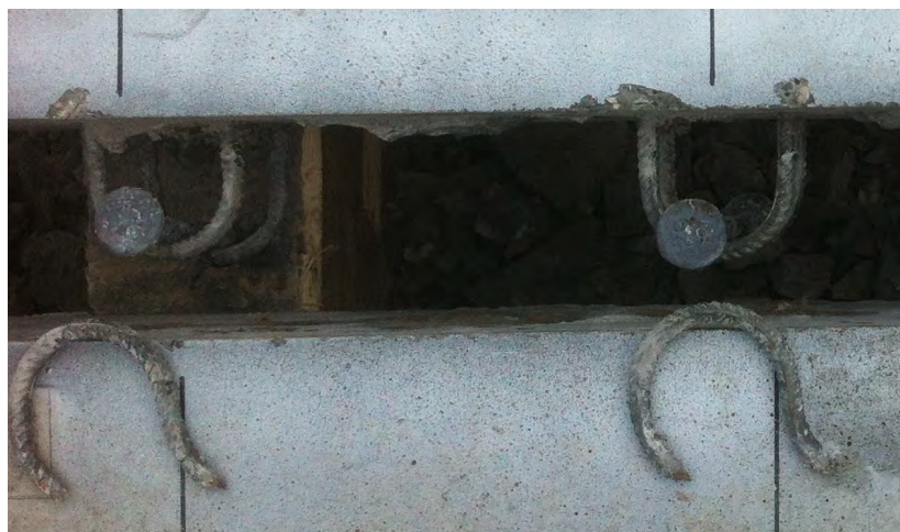
(c) New design '1-on-2' design (Specimen P12)
