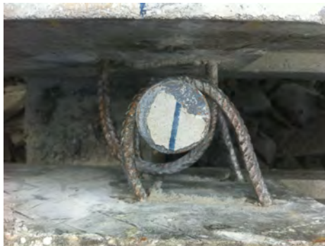
Figure 6.7: U-bar deformation observed with the new design, Specimen P2
