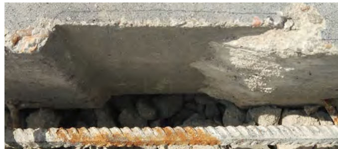
(b) Local key corner crushing, Specimen D12A
