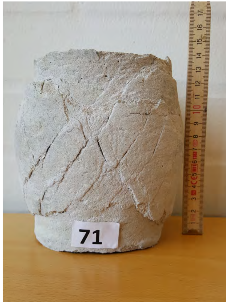
Figure 3.7: Example of highly deformed specimen from Mixture C2a
