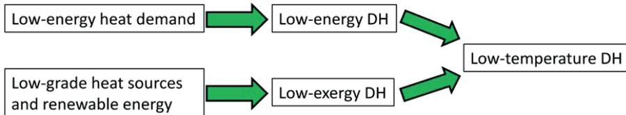
Figure 3.1 The low-temperature district heating concept.
