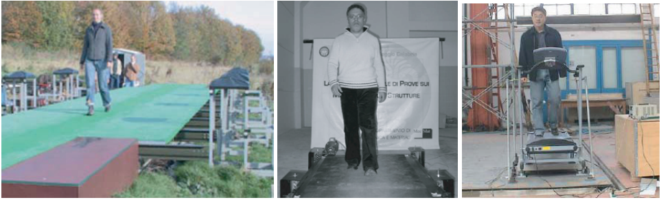
Figure 11: left: Laterally driven platform at RWTH Aachen (Picture from [8]). Middle: Laterally driven treadmill at the University of Reggio Calabria (Picture from [55]). Right: Instrumented treadmill on a shaking table at Tongji University (Picture from [31]).
