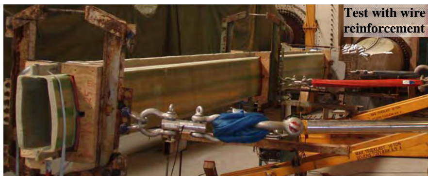
Figure 11. Photo of the second box girder test (test 3-5). The second box girder has also been shortened to 25.5m
