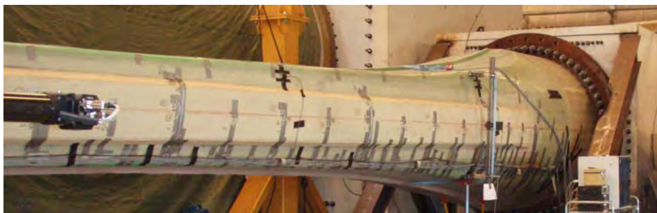
Figure 16. Tophat girder added to the first box girder structure to compensate for the removed aerofoil and eliminate an unrealistic buckling failure in the area (2-9m), where the removed aerofoil carries a large part of the flapwise loads due to the wide cord in this area.
