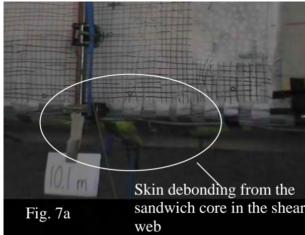
Figure 7: Failure observed at the shear web in the “new” box girder test a) Frozen frame picture showed skin debonding of the sandwich web towards leading edge b) Sketch which illustrate the failure and the strain gauges attached in that area.
