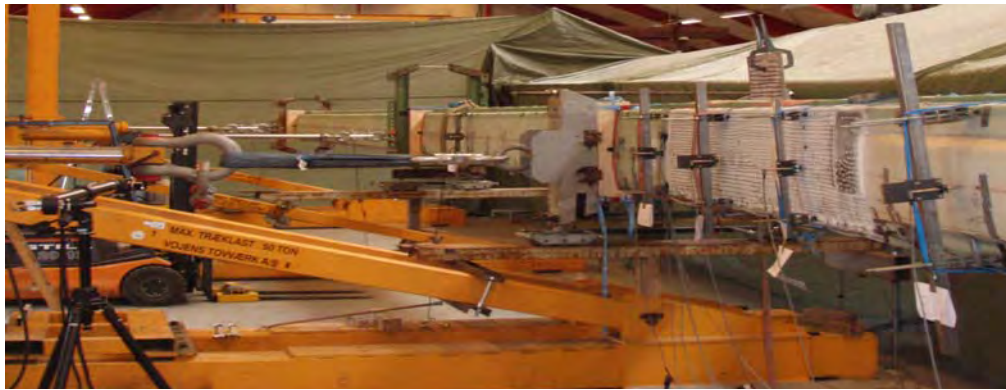
Figure 5: Full-scale test of 34m (shortened to 25m) load carrying box girder from SSP-Technology A/S, see ref. [4.] and [5.].
