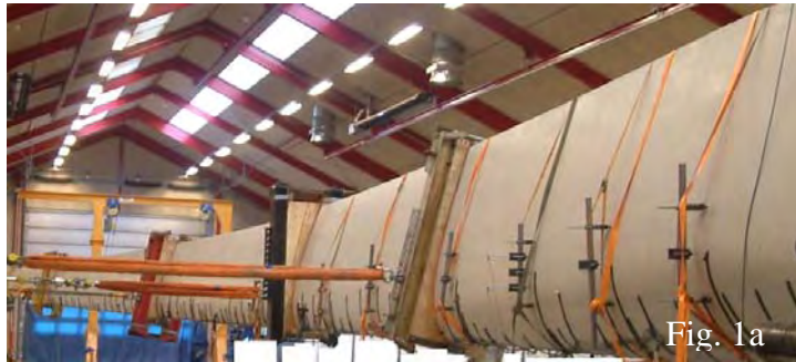
Figure 1: Full-scale test of a 34m blade from SSP-Technology A/S 1a) Photo from ref. [3.] 1b) Wind turbine blade subject to bending, leading to ovalization of the profile
