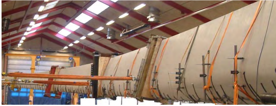
Figure 9. Photo of the first full-scale test of a 34m SSP-blade with extra measuring equipment.
