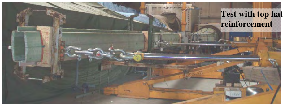
Figure 10. Photo of the first shortened 34m SSP-box girder (test 2). The box girder has been shortened to 25.5m.
