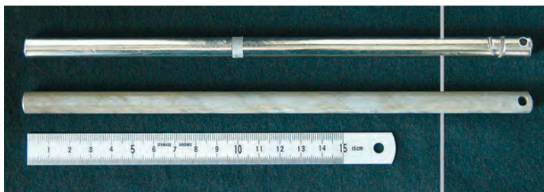
Figure 4.13 The two types of reinforcement bars prepared for the experiment. Lower: A cleaned and uncoated bar as used in Series I and II. Upper: A partly nickel coated bar as used in Series III. Only the length to the left of the vertical line was embedded in the test specimen.
