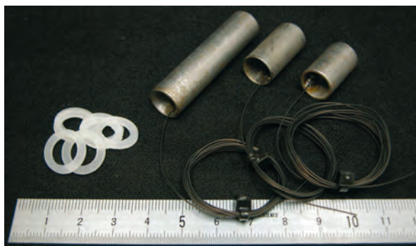
Figure 4.8 A wire is soldered to the inside of each segment, here with lengths of 20, 25 and 50 mm, respectively (from right). The silicone rings are placed between the segments when mounted on the fibreglass bar.
