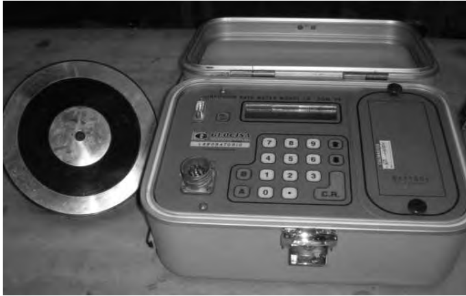
Figure 4.2 The GECOR 6 Corrosion Rate Meter from Geocisa, Spain (shown without connecting cables).
