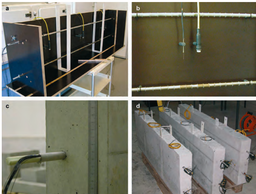
Figure 4.7 Manufacture of test slabs. a: Segmented reinforcement bars, reference electrodes, chloride sensors and lifting frames mounted in the mould (mould side removed for better view). b: All reinforcement segments are isolated with silicone rings. c: The fibreglass bar with the connecting wires and a part of the 160 mm end segment protruding from the slab. d: The three test slabs - ready for testing.
