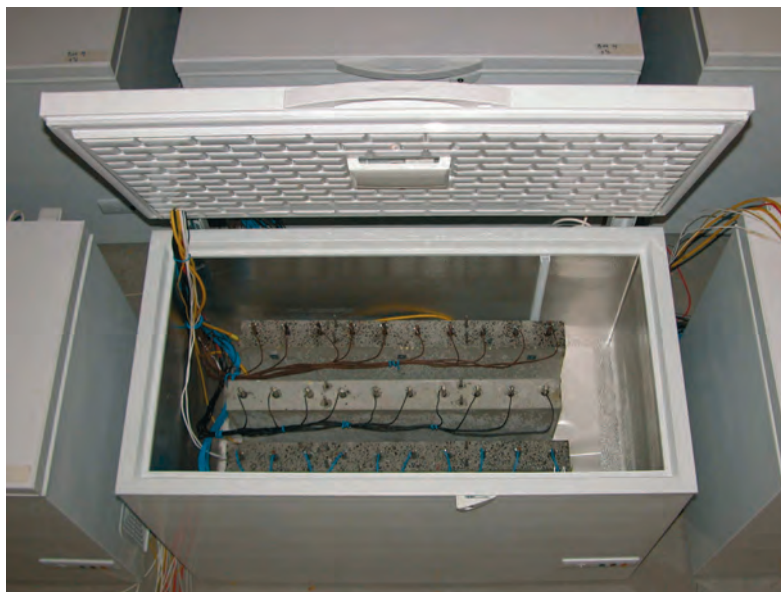
Figure 4.14 A test specimen from each series (I-III) is placed in each climate chamber maintained at a constant temperature and relative humidity.
