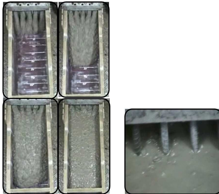
Figure 7.30 Photos from testing mix E_1 in the L-box test with reinforcement setup A_{lbox} .
