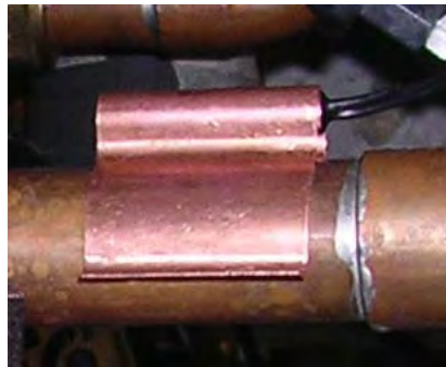
Fig. 5–8 Advanced standard sensor based on a NTC element in a copper cylinder with a copper clamp to be clipped on a pipe.
