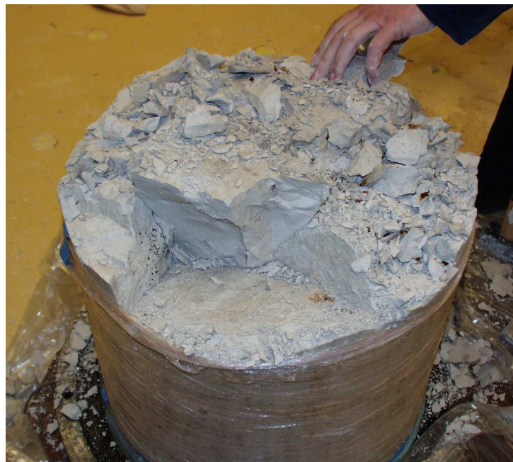
Figure L.5 Disassembling of specimen 8 by use of a hammer and a chisel.
