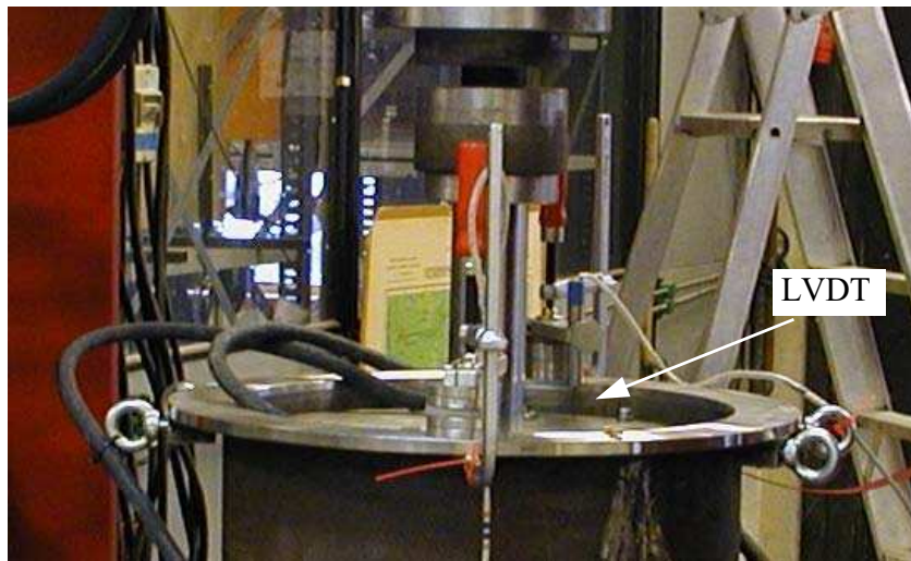
Figure N.4 Two LVDTs placed opposite each other on top of the oedometer cell treading down on the load piston. The arrow points to one of the LVDTs
