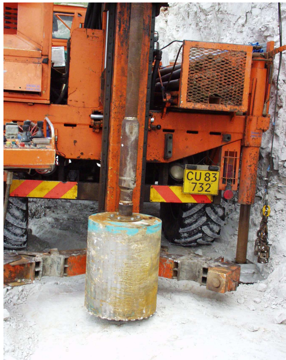
Figure C.7 The drill bit is mounted on the drilling rig.
