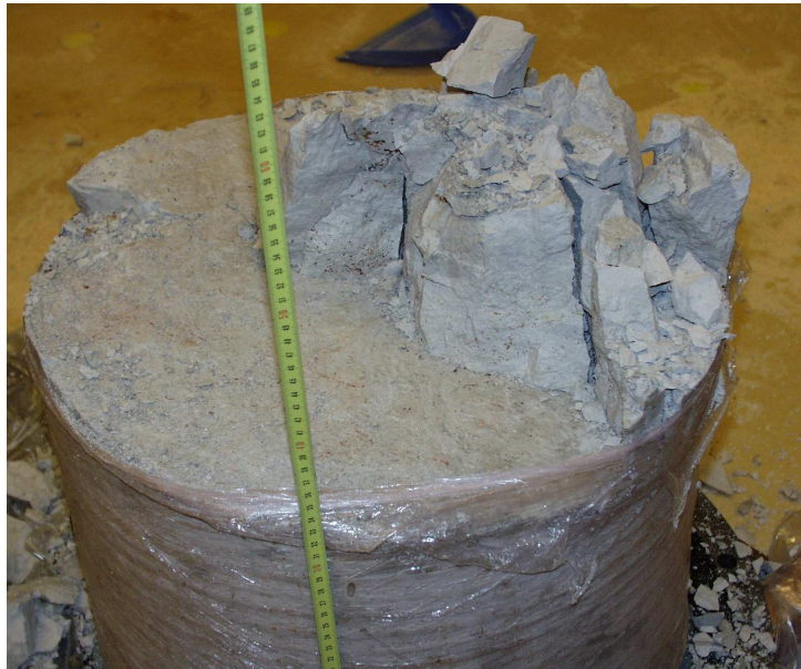
Figure L.6 The upper of the two horizontal fracture planes in specimen 8 after test.
