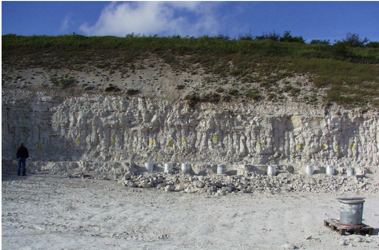
Figure 5.1 View of the wall and the bench. The chalk is removed around most of the twelve specimens, which are wrapped in metal shields. In the front, the first sampled specimen is seen.
