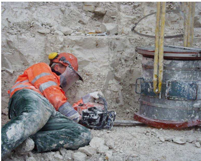
Figure C.13 The specimen is cut free at the bottom by use of a chain saw.
