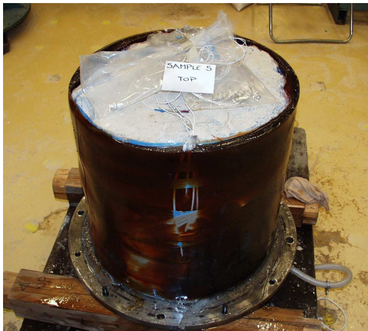
Figure L.3 Specimen 5 after test. The membrane has been removed, and the rubber cast around the specimen is seen.
