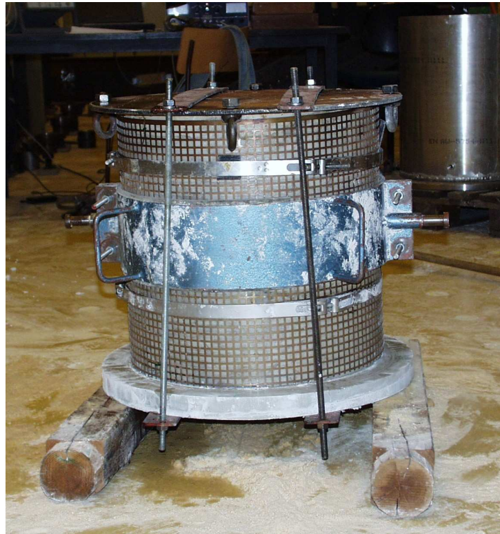
Figure 5.2 A specimen equipped with a lifting arrangement for turning the specimen upside down in the laboratory.
