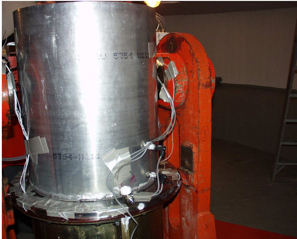
Figure 6.8 Photograph of leads from the TDR probes and the PPTs secured with tape and strips before centrifuge testing in the new test set-up.
