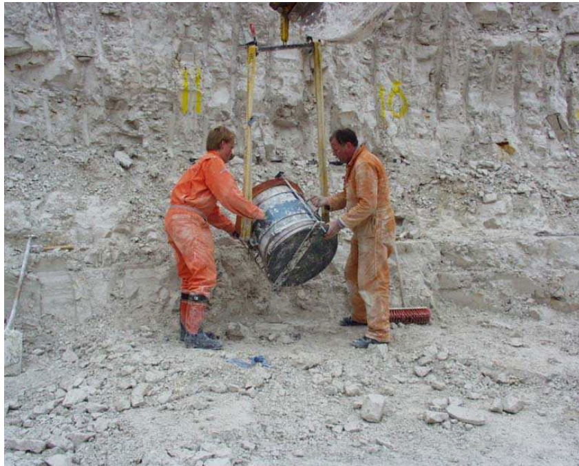
Figure C.14 The specimen is turned upside down for a rough trimming of the bottom.
