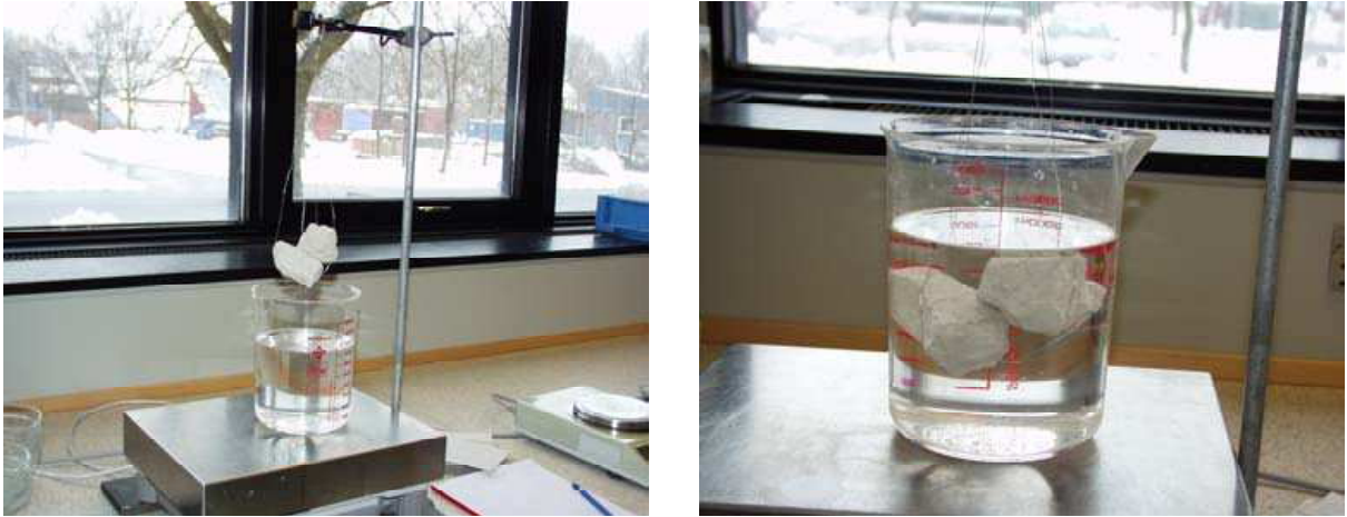
Figure 6.24 Photo of the set-up for measuring the submerged weight of the small samples.
