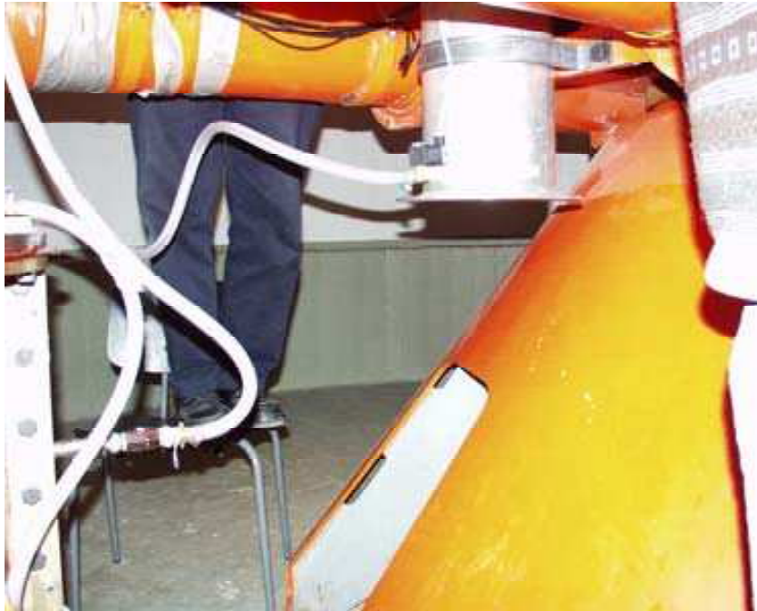
Figure 6.3 Photograph of the additional container mounted near the centrifuge axis.
