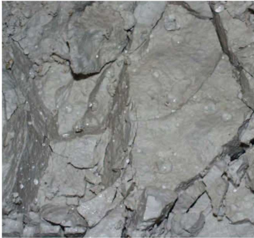
Figure 5.4 Photograph of the fractional-wet specimen 2 after test with drops of water on the oil-wet surfaces.
