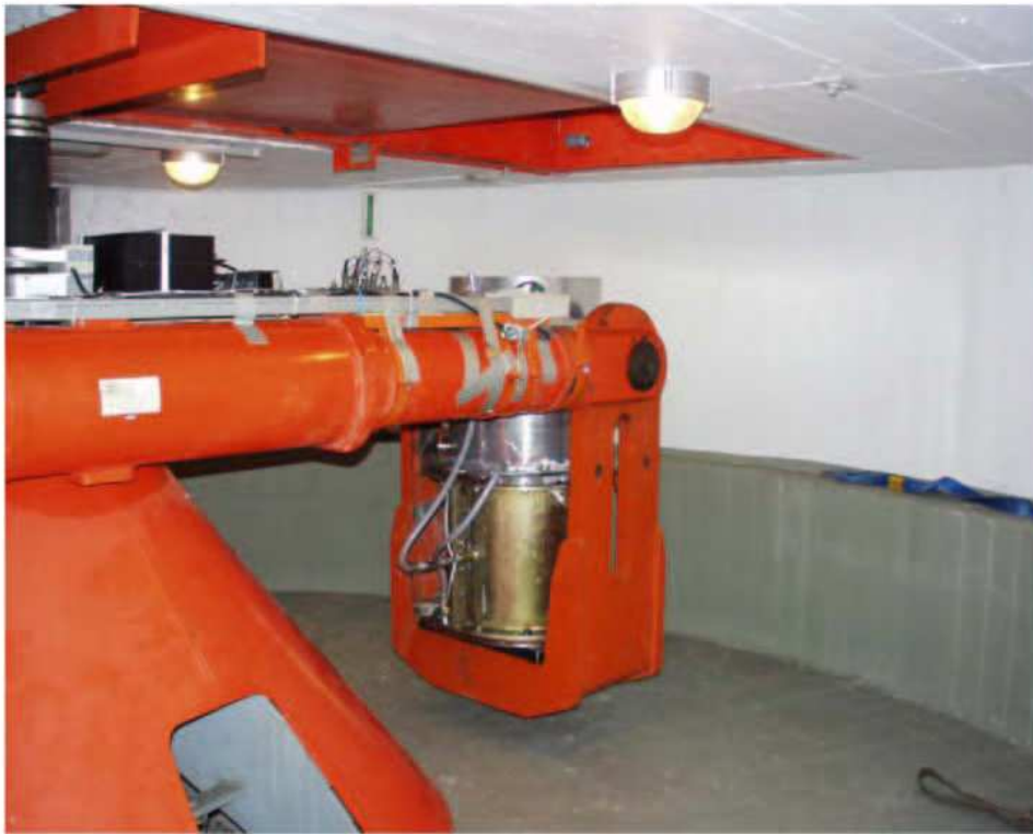
Figure 6.7 Photograph of the new test set-up mounted in the centrifuge.
