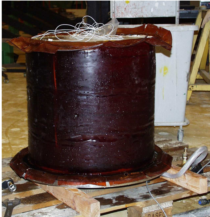
Figure L.2 Specimen 8 after test. The form is removed, but the membrane is still on the specimen.
