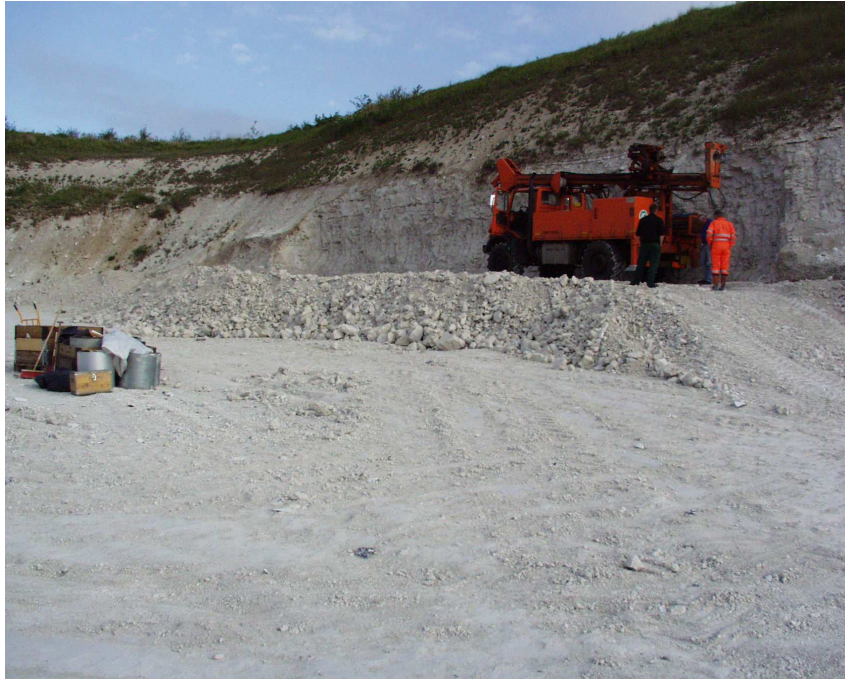
Figure C.6 The mobile drilling rig on the chalk bench.
