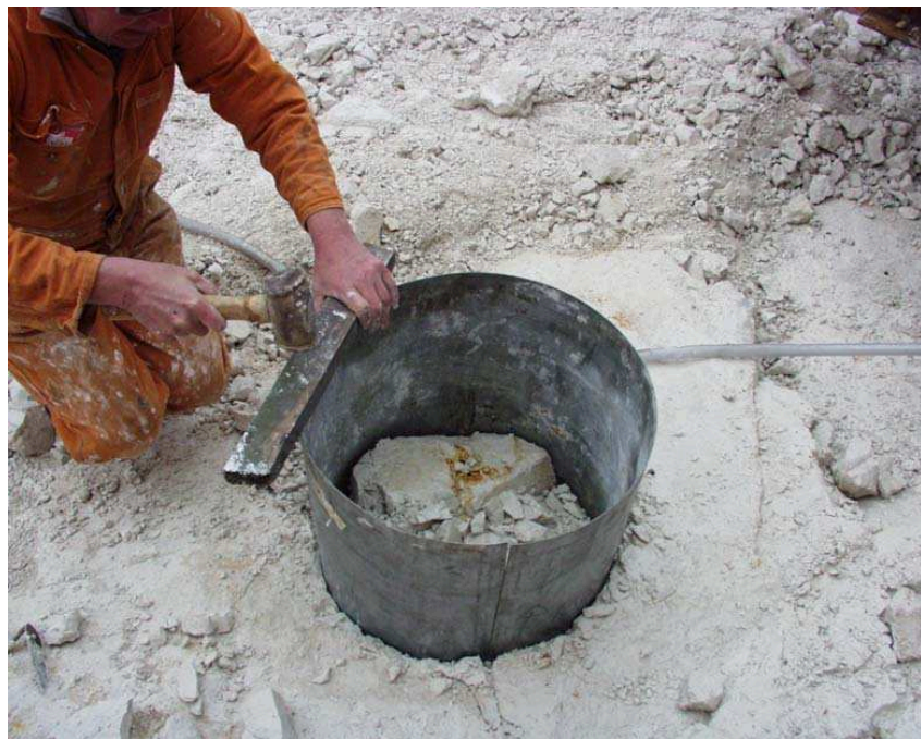
Figure C.9 Insertion of metal shield in the drill bit trace.
