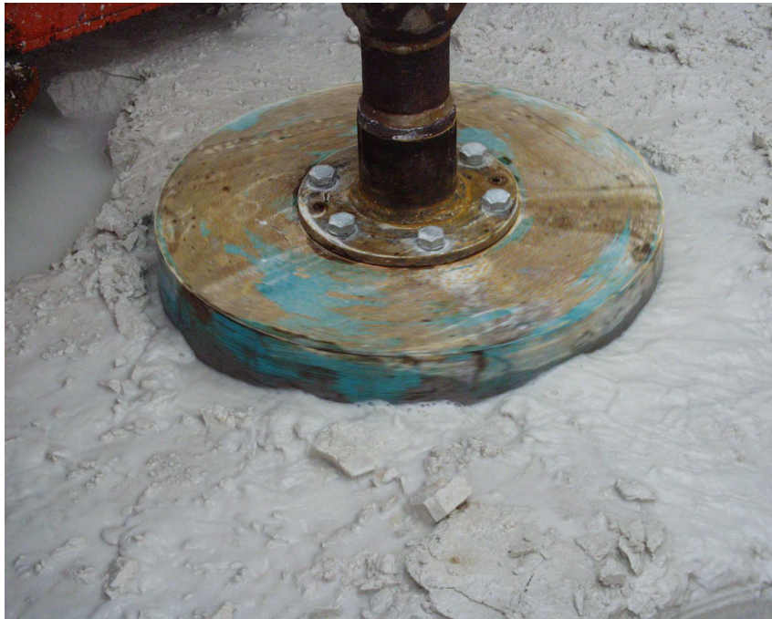
Figure C.8 Water was used to cool the drill bit and flush away cuttings during drilling.
