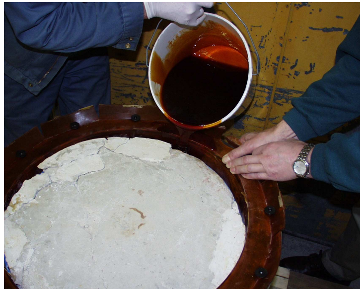
Figure J.5 Liquid rubber mass is poured into the excess space between specimen 11 and the rubber membrane.
