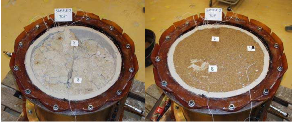
Figure 5.3 Specimen 2 with the ring of gypsum (left) and the layer of sand laid out within the ring of gypsum (right). The specimen is instrumented with TDR probes.
