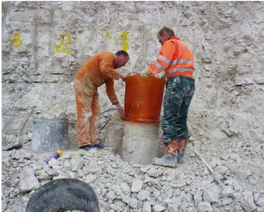
Figure C.12 A rubber membrane is pulled over the specimen.
