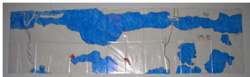
Figure G.7 Fractures (black lines), voids at the surface (red) and gypsum (blue) indicated on plastic for specimen 10.
