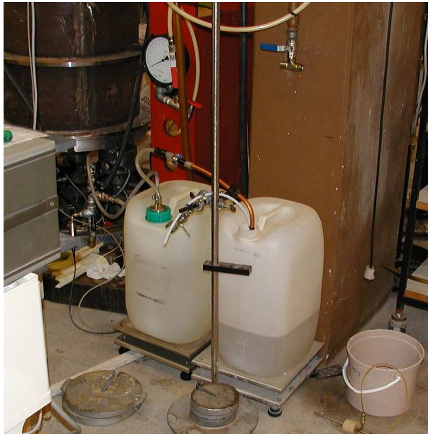
Figure N.1 Displaced fluids recorded on a double-balance system.
