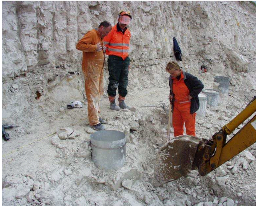
Figure C.10 Rough excavation in front of and beside the specimen performed by use of the backhoe. The excavation is supervised to prevent fracturing.
