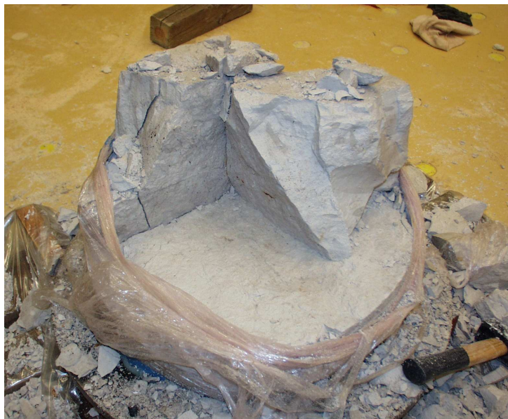
Figure L.7 The lower of the two horizontal fracture planes in specimen 8 after test.
