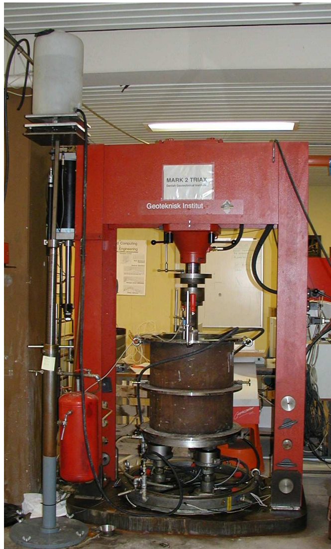
Figure 8.2 Photo of the oedometer cell mounted in the MARK-2 set-up. The inlet container is seen elevated to the left.
