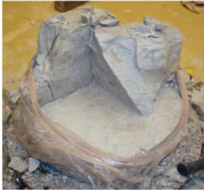
Figure 5.6 Photograph of the lower of the two horizontal fracture planes in specimen 8 after test.
