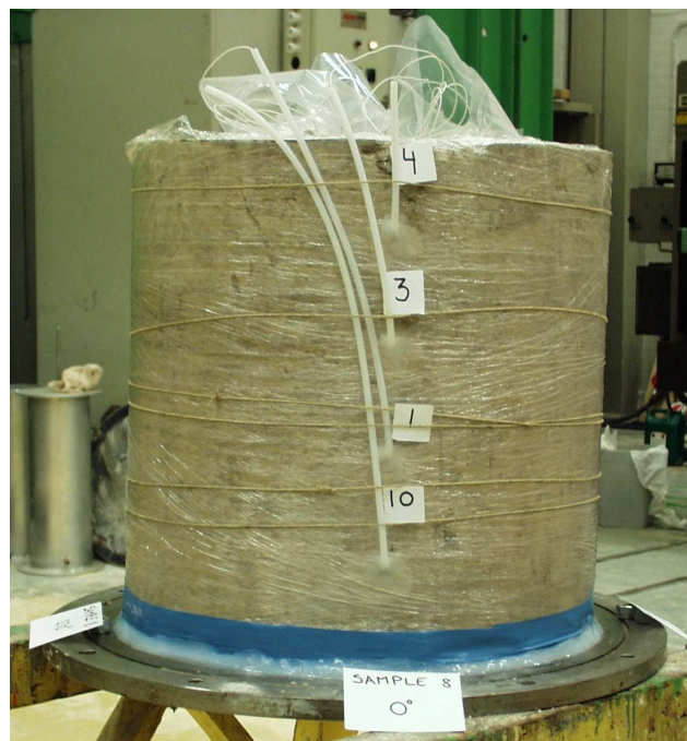
Figure J.3 Specimen 8 wrapped in soft plastic foil. Silicone sealant is seen along the periphery of the specimen at the bottom plate. TDR probe 1, 3, 4 and 10 are mounted in the specimen. The probe leads are secured with safety tubes, which are taken along the specimen to the top. The holes are sealed with silicone sealant.
