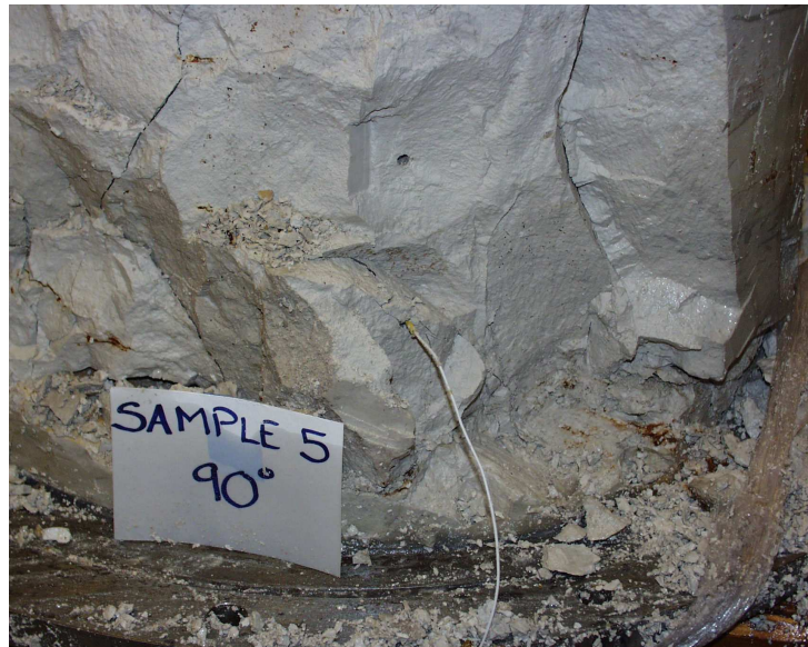
Figure L.8 TDR probe in specimen after testing.
