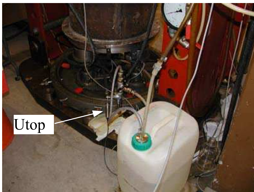
Figure N.3 Outlet pore pressure transducer, Utop .
