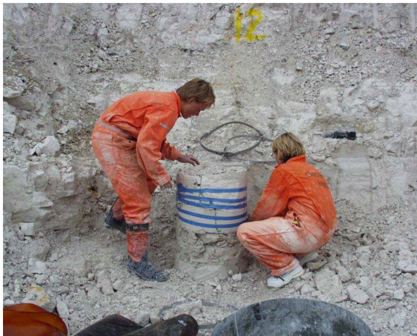
Figure C.11 Blue tape wrapped around the specimen to keep the fractured specimen together.
