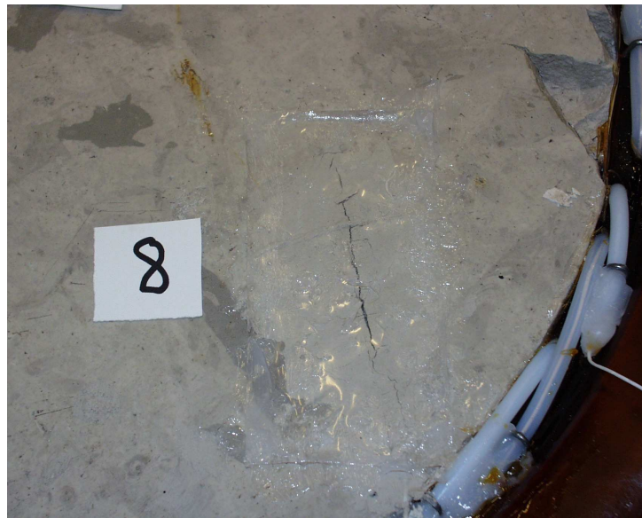
Figure J.6 Horizontally placed TDR probe down into the matrix part of the specimen 8 top. The probe is covered with a mix of pulverized chalk and Isopar-L, and covered with plastic fastened with silicone grease.
