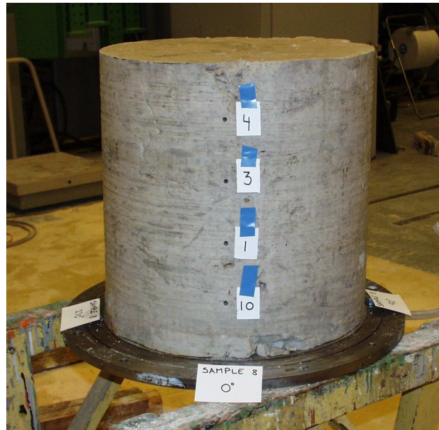
Figure J.2 Specimen 8 with holes drilled for TDR probe 1, 3, 4 and 10.
