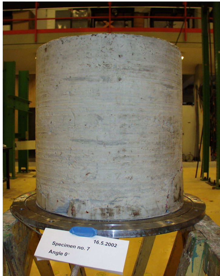
Figure J.1 Specimen 7 placed on the porous filter on the bottom plate.
