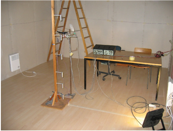
Figure 6.21 Room. Four 500W heating panels (two can be seen here) are installed on each wall. Centrally in the room, measurements of temperatures (air, radiant and operative) are performed as well as air velocity and relative humidity.
