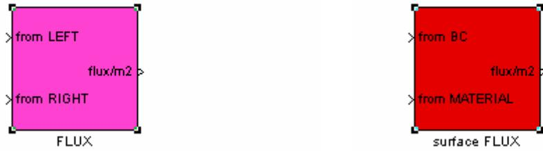
Figure 17: The **flux** and **surface flux** block. Input is the data arrays from the nodes, one wants to define the flux for. Output is a flux density. The unit of the flux depends on the time defined for integration.
