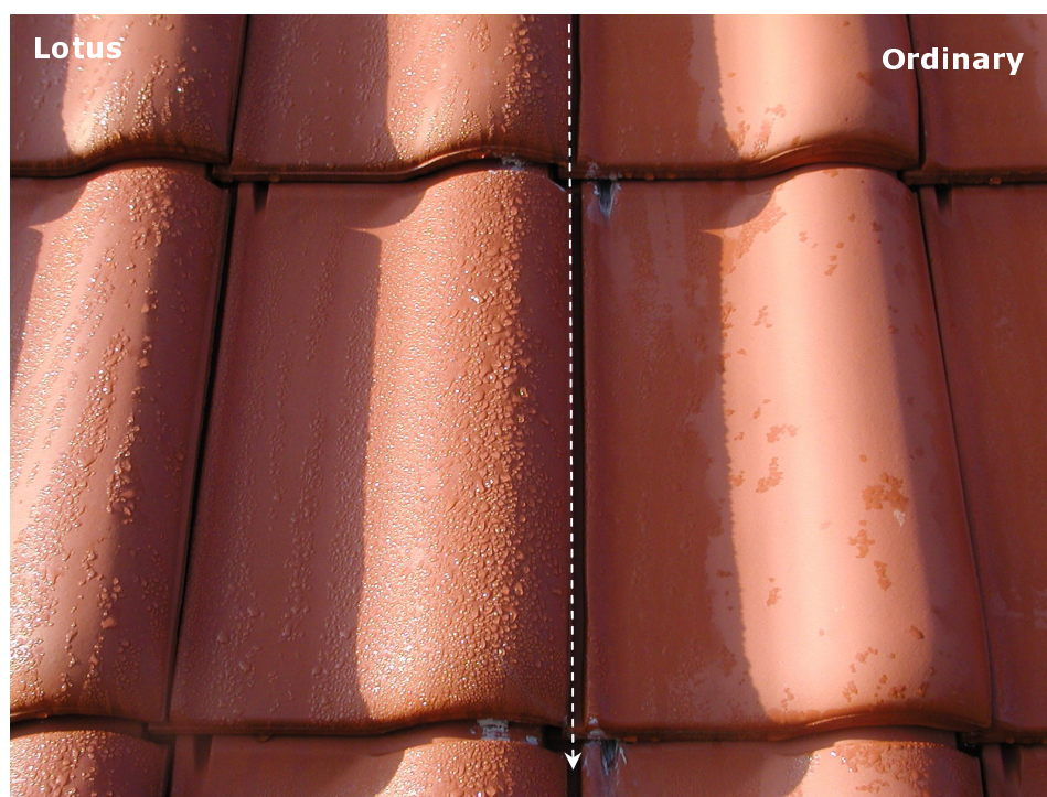
Figure 5.23: Dew at tiles. Left: Dew forms droplets at tiles with Lotus Effect. Right: Dew is only visible as a film on ordinary tiles or has already dried up.
