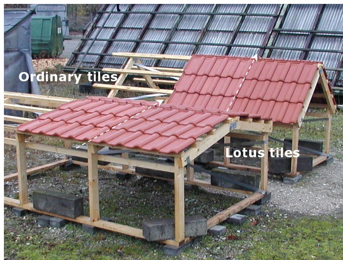
Figure 5.1: The set-up at DTU. Tiles with Lotus Effect are placed at the eastern side of each roof. In this and the following pictures from the set-up are the tile types divided by a dashed line with an arrow facing north.
