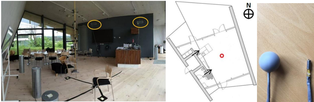
Fig. 7. Panoramic view of the interior (left), the measurement location (middle) and the globe and air temperature sensors (right).
