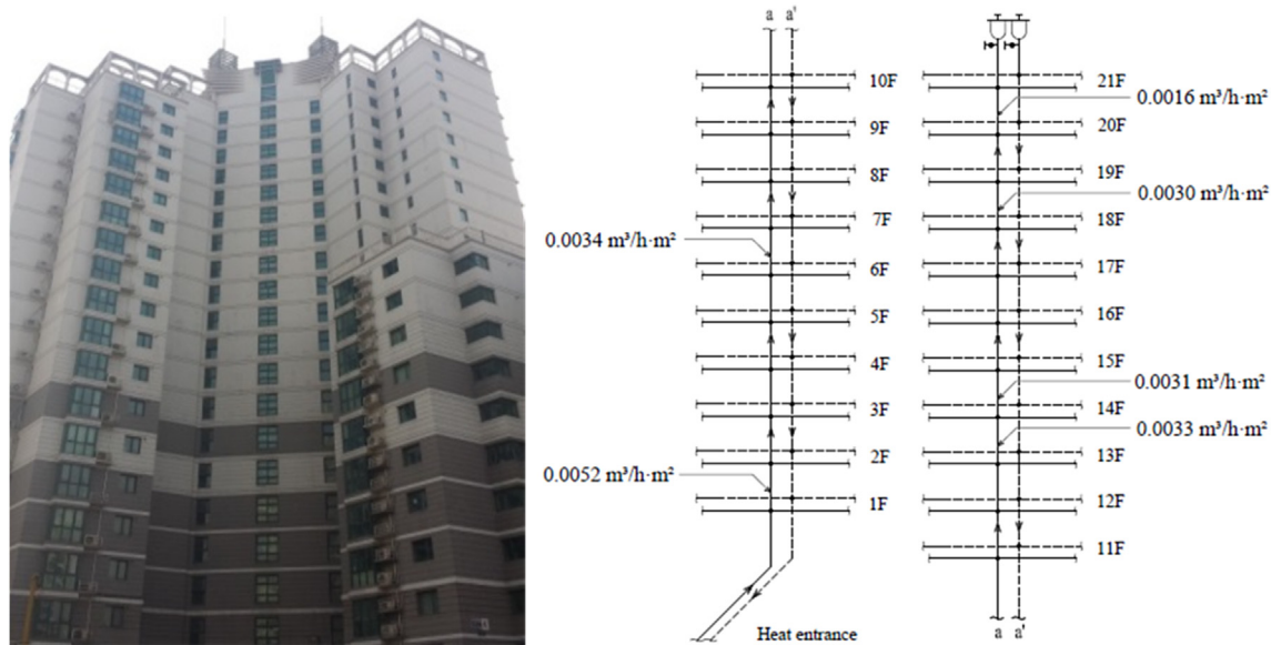
Fig. 3. Flow measurement of a high-rise building in Beijing.
