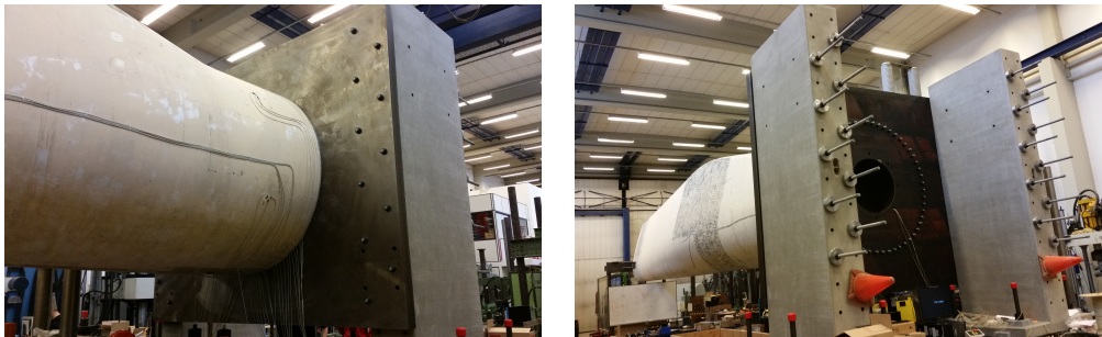
Figure 1.7: Installation of Wind Turbine Blade Root on Strong Wall, January 2016, DTU Byg.
