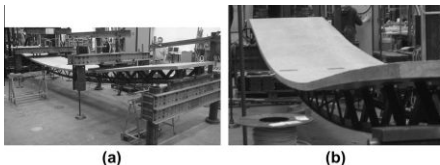
Fig. 20. Deformed shape of specimen MP2 during (a) and after (b) ULS loading.
