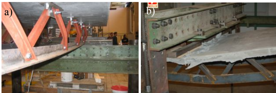
Figure 6-10 a) Buckling of compression diagonals in specimen MP1, and b) A combination of compression and flexural failure during ULS testing of specimen MP4.
