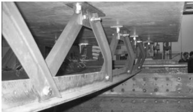
Fig. 19. Buckling of compression diagonals in specimen MP1.
