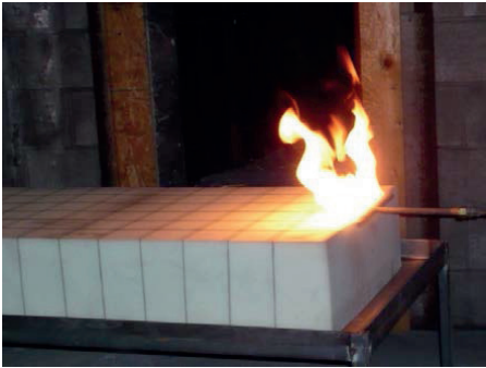
Figure A1. Ignition of PUF block with a 19 kW propane T-burner.
