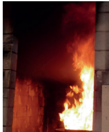
Figure 6. Measured vertical temperature distribution at TCT 1 at time of ignition of the crumbled paper (lining 1; 2 min and lining 2; 7 min) and photo illustrating the division of layers.
