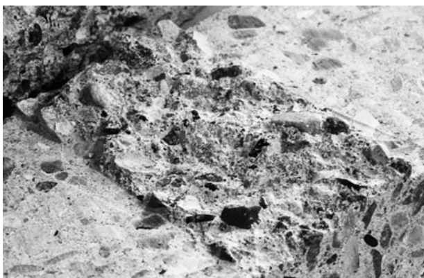
Fig. 11 Close view of the crack surface for the 40° mixed mode test
