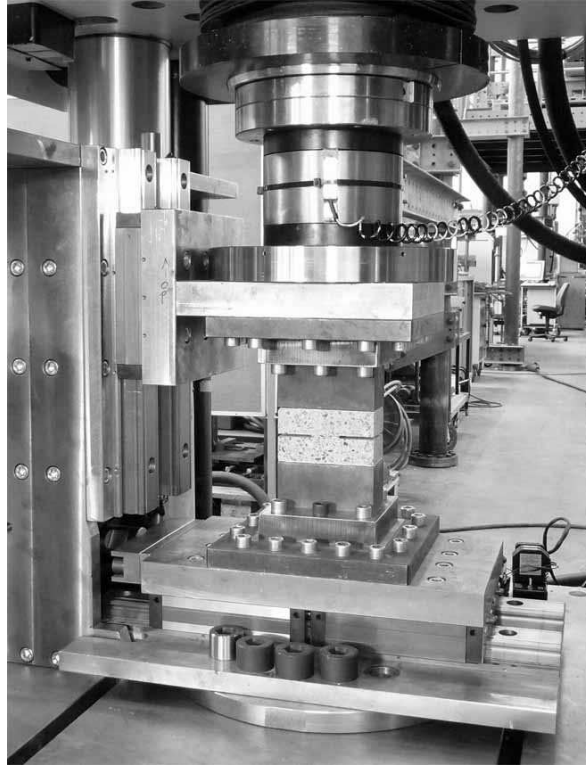
Figure 3.4: Test set-up with a glued in specimen. The photo shows the vertical load cell, the support structure and the slides in both vertical and horizontal direction.
