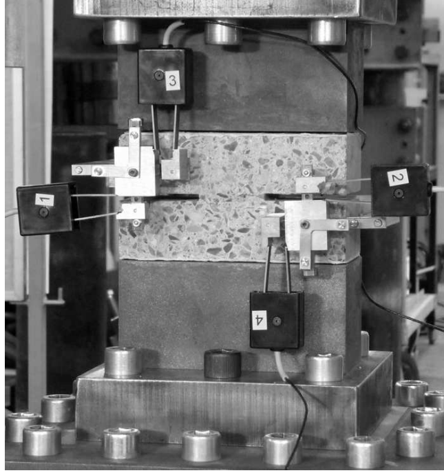
Figure 3.10: Close view of test specimen, gauges rails and clip gauges.
