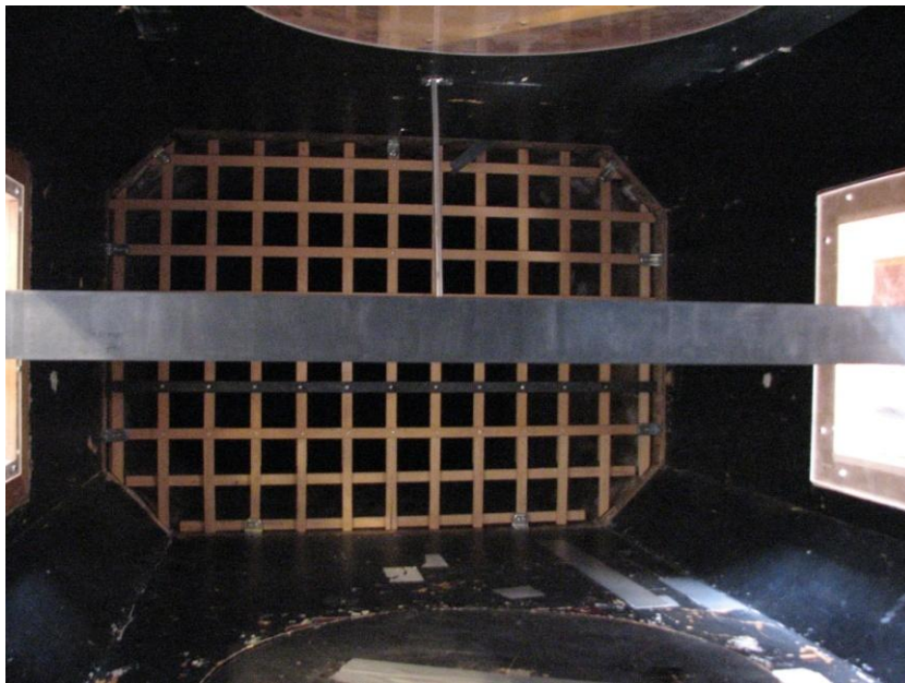
Figure 33. D-section Model Mounted in Wind Tunnel, Turbulent Flow
