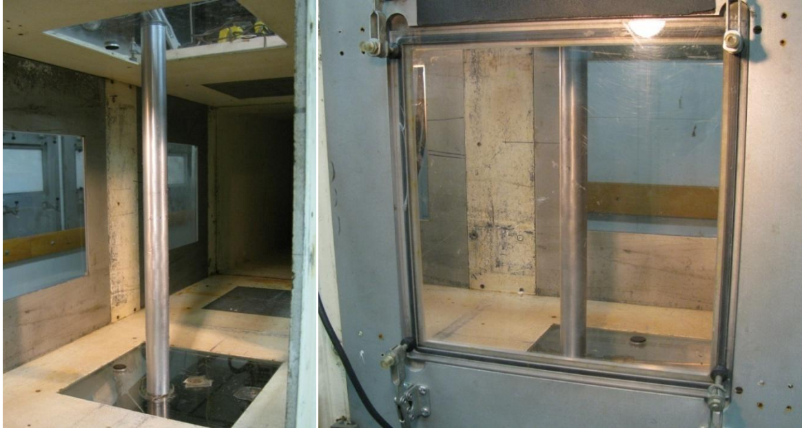
Figure 6 Arrangement of vertically mounted small cylinder in the test section centre.
