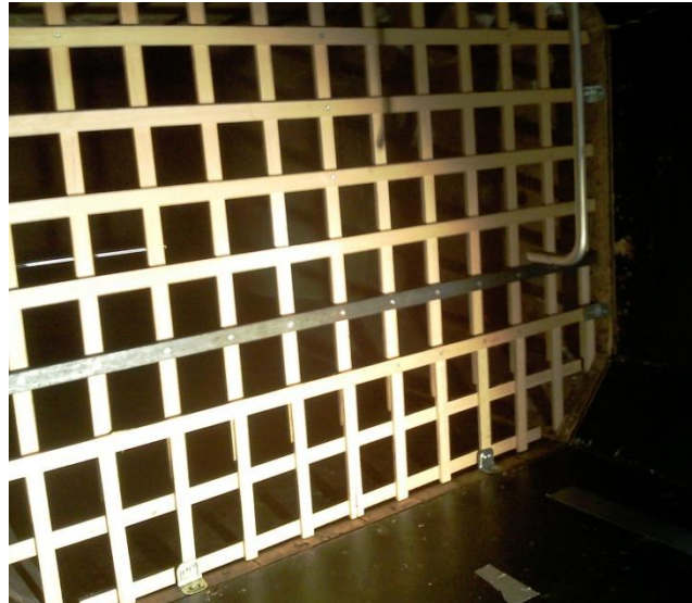
Figure 26. Picture of Turbulence Grid and Pitot Tube Location.
