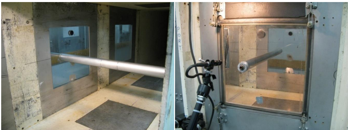
Figure 5 Arrangement of horizontally mounted small cylinder in the test section centre.
