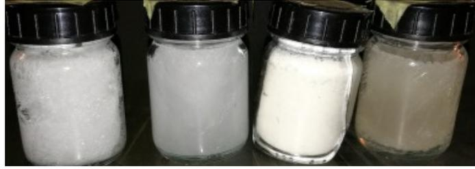
**Fig. 1. SAT composite samples after crystallization (from left: SAT, SAT + water, SAT + CMC, SAT + HD 310).**
