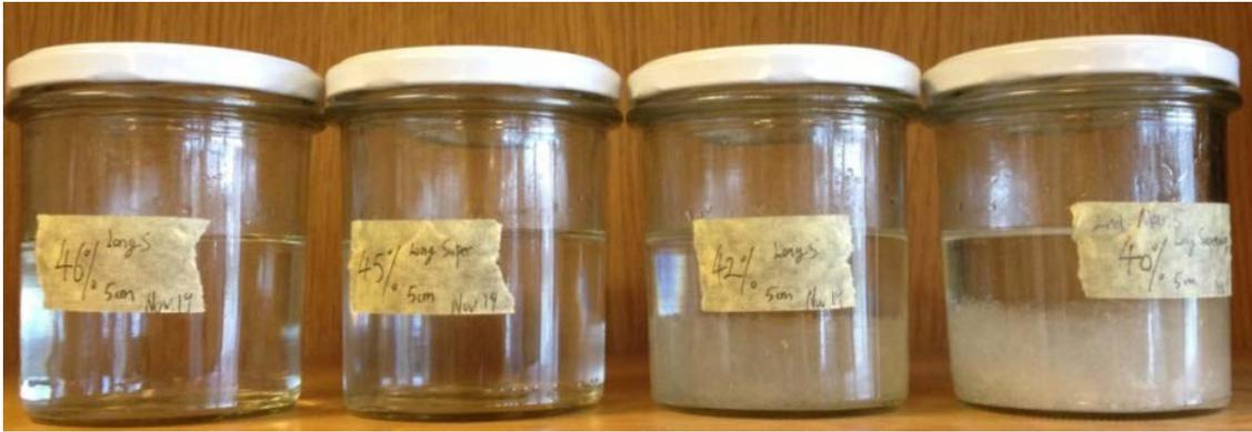
Fig. 6 The 40%, 42%, 45% and 46% salt water mixtures from right to left after 100 days supercooling
