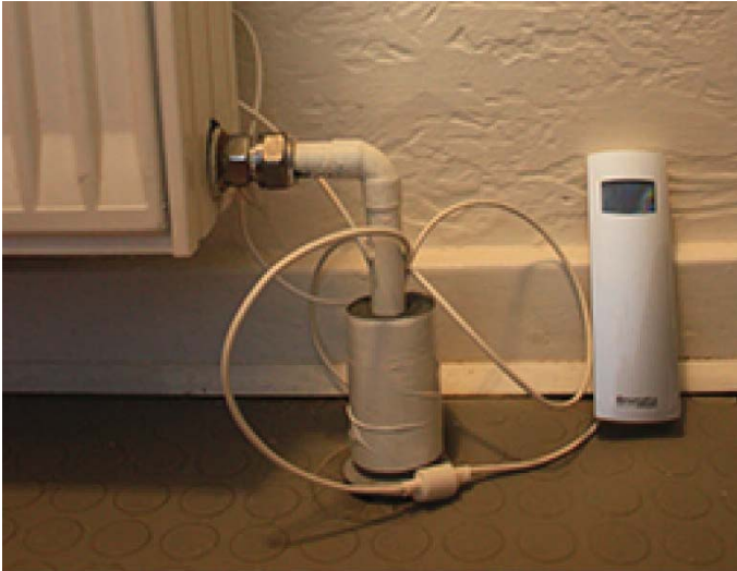
Fig. 9. Temperature measurements on the radiator return pipes in some of the houses (Paper V)
