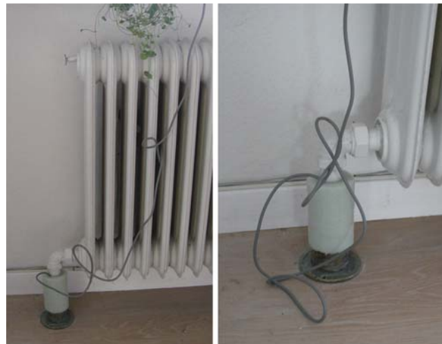
Fig. 4. Pictures of the measurement setup. The pictures illustrate the mounting of the temperature probe to the outlet pipe of the radiator.
