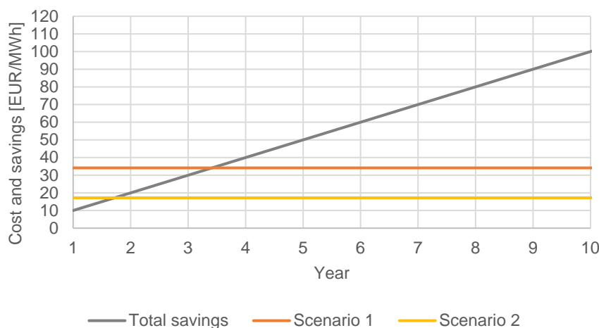
Fig. 25 Simple pay-back time of the two scenarios for investments to prepare existing space heating systems for low-temperature district heating (Paper VIII)
