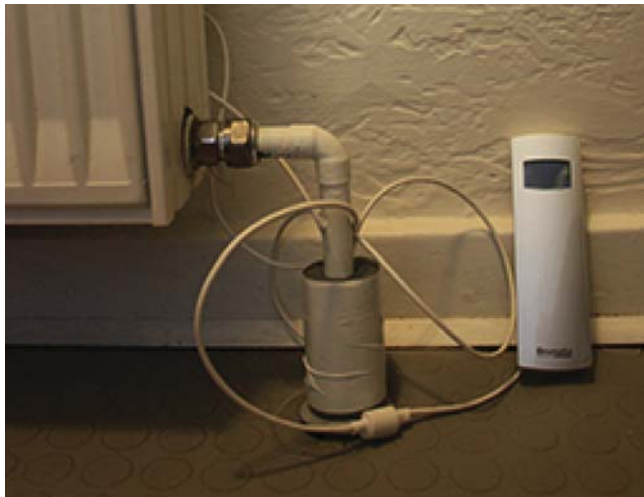
Fig. 3. Equipment setup for the measurement of return temperatures from radiators.
