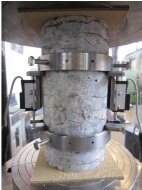
Fig. 3: Test setup for the uniaxial compressive test. The deformations during loading were measured by two LVDTs placed between rigid rings closely fixed to the concrete core.
