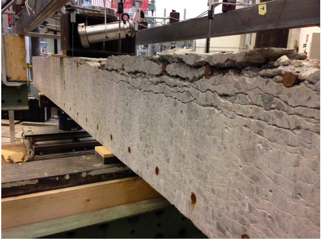
Figure 4: Local increase in crack widths in compression zone of a beam from segment 6 due to combined effect of ASR and corrosion.
