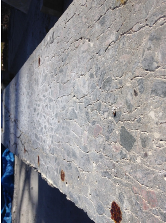
Figure 3: Typical ASR crack pattern on the section of segment 5.
