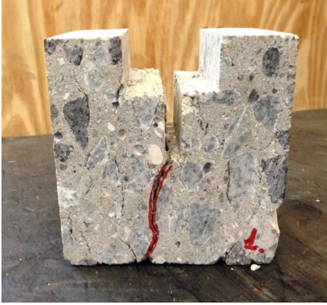
Fig. 12. WST cube with orientation I after testing. The ASR cracks were opened due to the splitting load.
