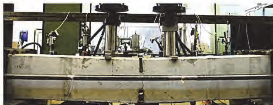
Fig. 9. Example of possible post-tensioned full-scale concrete hinge for PC arches being tested at the Technical University of Denmark.
