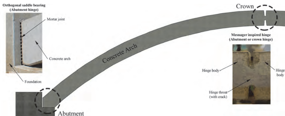
Figure 4: The two types of investigated hinges for PC-Arches. The Mesnager hinge can be used as abutment hinge as well as crown hinge.
