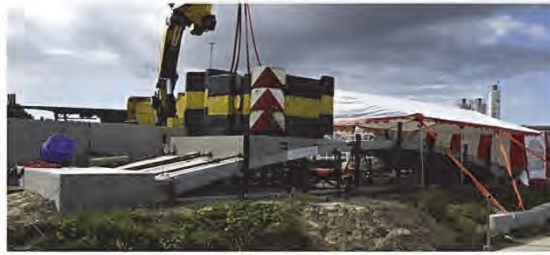
Fig. 11. Test of two PC arches with 66 tons of load in the critical 1/4 point of the span.
