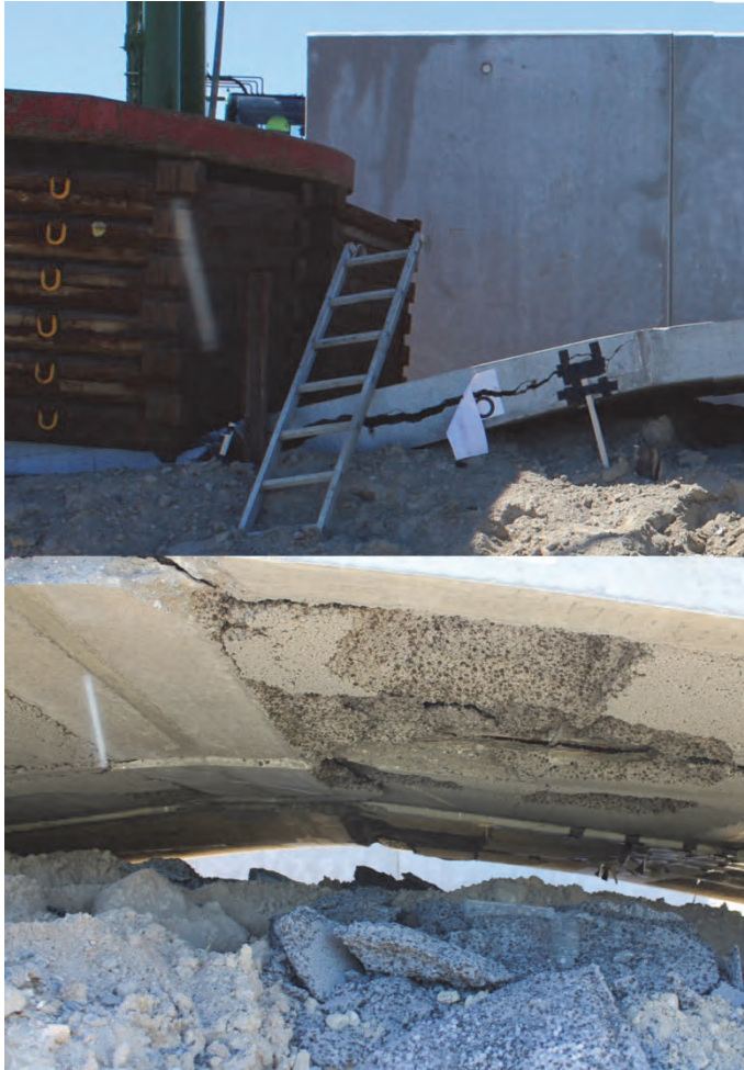
Figure 20: Photographs taken after collapse: longitudinal crack at 3/8 point (top) and crushed concrete at 5/8 point (bottom).
