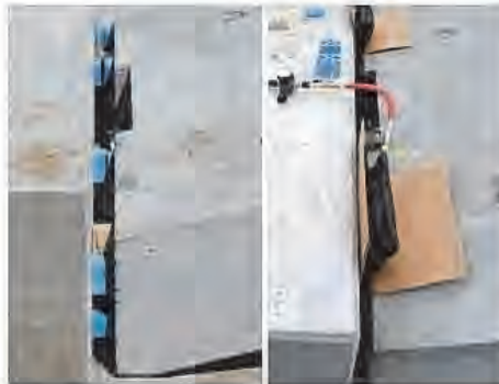
Fig. 5 Connection detail between foundation and arch. Left: First PC test arch was connected by plastic pieces and wood wedges. Right: Second PC test arch was connected by pumping up hydraulic flat jacks (requiring 6 bars of pressure).
