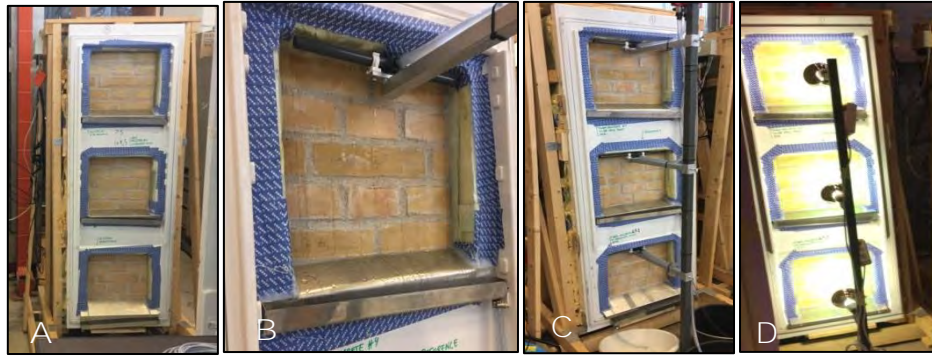
Figure 19: Experimental setup. A: 3 wall sections mounted in a refrigerator door. B: water loads applied horizontally to the top of the wall section, by perforated pipe. C: view of water loads applied to 3 wall sections. D: radiation loads on 3 wall sections.
