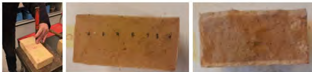
Fig. 3. Halving of brick specimens with hammer and chisel (left), marking of 7 measuring locations on both sides (agent L), and example of visible penetration depth, the lighter area around the brick (agent E).
