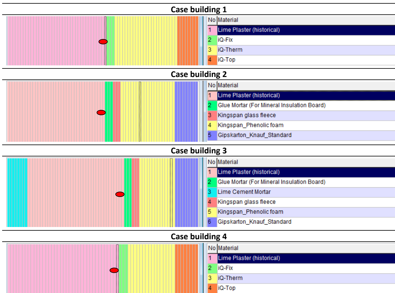
Figure 15: 1-dimensional simulation models (Delphin) for the four case studies. Discretization causes the formation of layer thicknesses not being representative in the images. Output locations are marked with a red dot.
